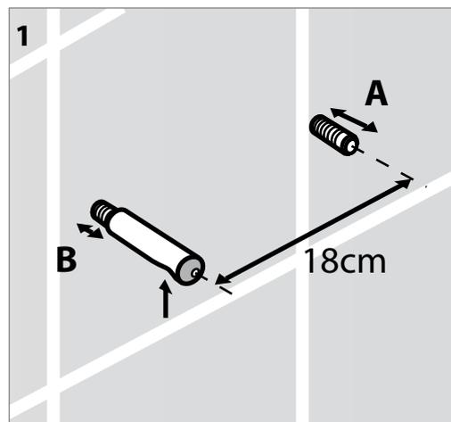
**2** Prepare the connection for the outlet pipe to the correct dimension shown. Assemble the outlet connection on the WC and cut it according to the correct length. Then locate the WC on the fitting bolts and push it to the wall taking care to correctly engage each connection. Applying a suitable silicone lubricant prior to final install will assist.
