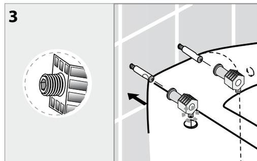
**4** Fully tighten the fitting screws using the key supplied, make sure the WC is screwed flat to the wall surface. We suggest to rotating the screw fixing little by little until the WC is securely fitted.
