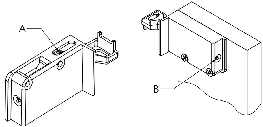
You may need to increase the length of the hook's protrusion. To do so turn screw 'B' anti-clockwise.
