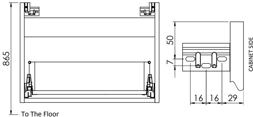
Fix Wall Hanging Plates as shown above. Check the type of wall you are fixing to and use the suitable fixings. (Not supplied).
