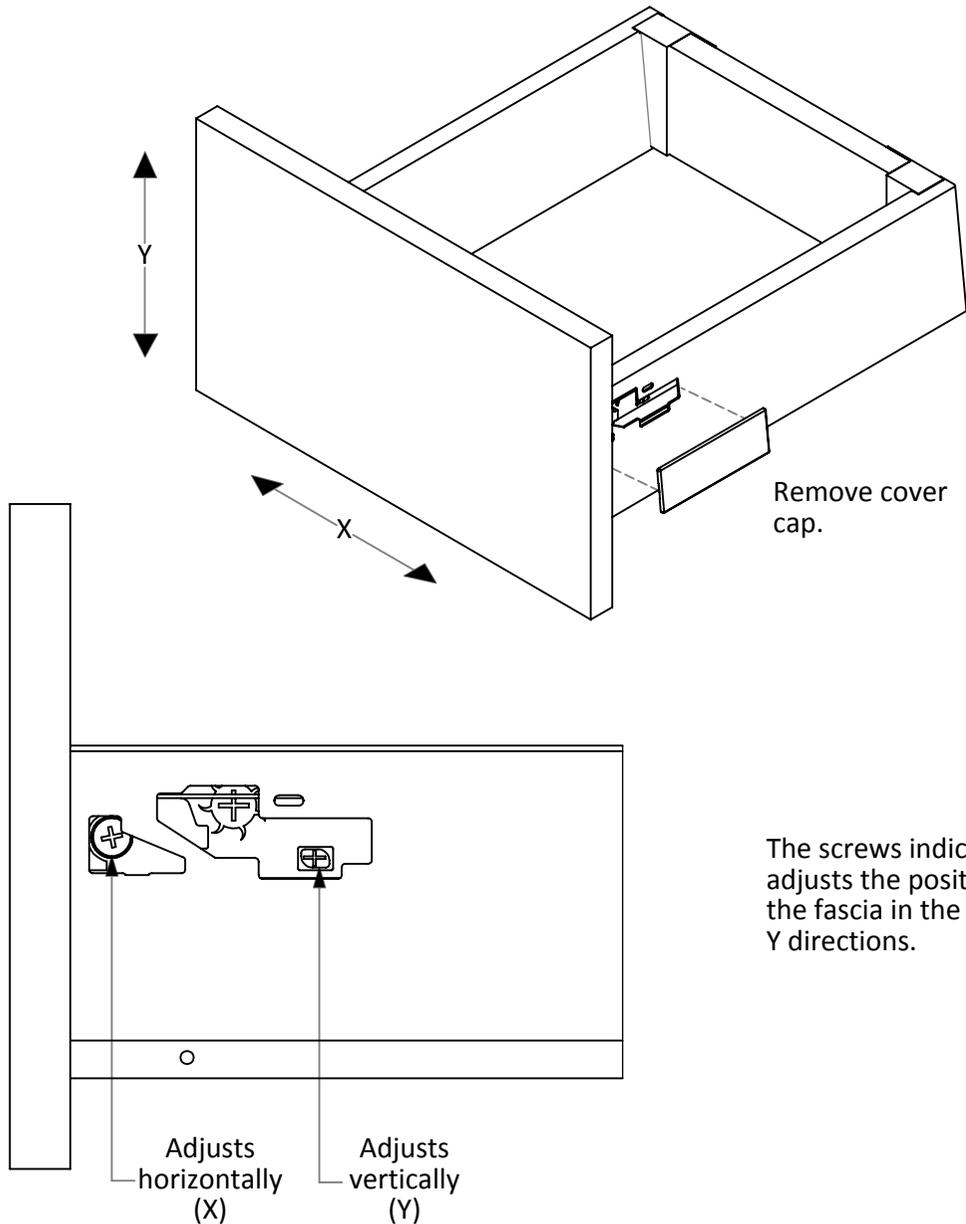
The screws indicated adjusts the position of the fascia in the X and Y directions.
