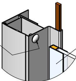
SLIDE THE CONCEALED MAGNET (ITEM 11) INTO THE PROFILE. CHECK POLARITY ATTRACTS DOOR BEFORE INSERTING. FIT DOOR MAGNET ITEM 12 TO DOOR GLASS.
