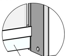
FIT THE DOOR BOTTOM SEAL (ITEM 14). IT SHOULD BUTT UP TO THE VERTICAL PROFILE WITH THE HINGES ON. CUT TO LENGTH FIRST BEFORE FITTING. THE SIZE IS AS FOLLOWS;
