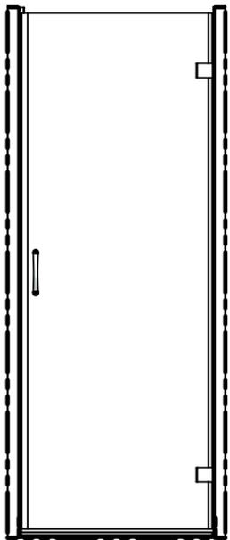
EXTERNALLY SILICONE SEAL THE WALL PROFILES WHERE THEY MEET THE WALL AND ALONG THE BOTTOM WHERE THEY MEET THE TRAY. ALSO FULLY SEAL THE DRIP STRIP AND RETAINER CLIPS (ITEM 4 & 15) ALL IN A CONTINUOUS BEAD.
