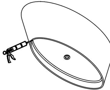
Attach waste fittings and fix your bath using white/clear bath sealant which must be applied to the bottom face of the bath. Clean off excess and be careful not to over-silicone.
