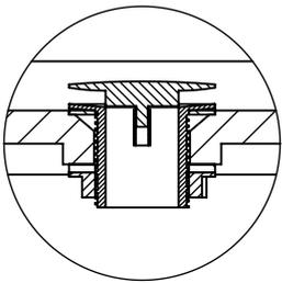
Insert the 'Push Button Waste' through the aperture and seal it in place using a silicone sealant. **DO NOT OVERTIGHTEN** the Backnut as this may cause the bath to crack.
