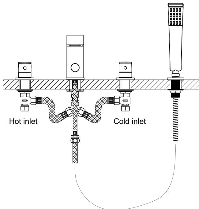
Connect the tee connector and the hot/cold control valves using braided hoses. Connect one end of the shower hose to the flexible tail of spout assembly and the other end to the shower, ensuring a washer is in. Adjust all parts in their position and then tighten all connections. Connect water supplies and the hot/cold control valve. Check for any leaks.
