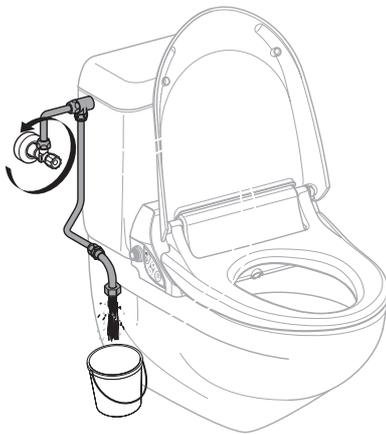
**7** Close the angle stop valve again, turn the connection bend upwards and connect it to the AquaClean 4000 shower toilet
