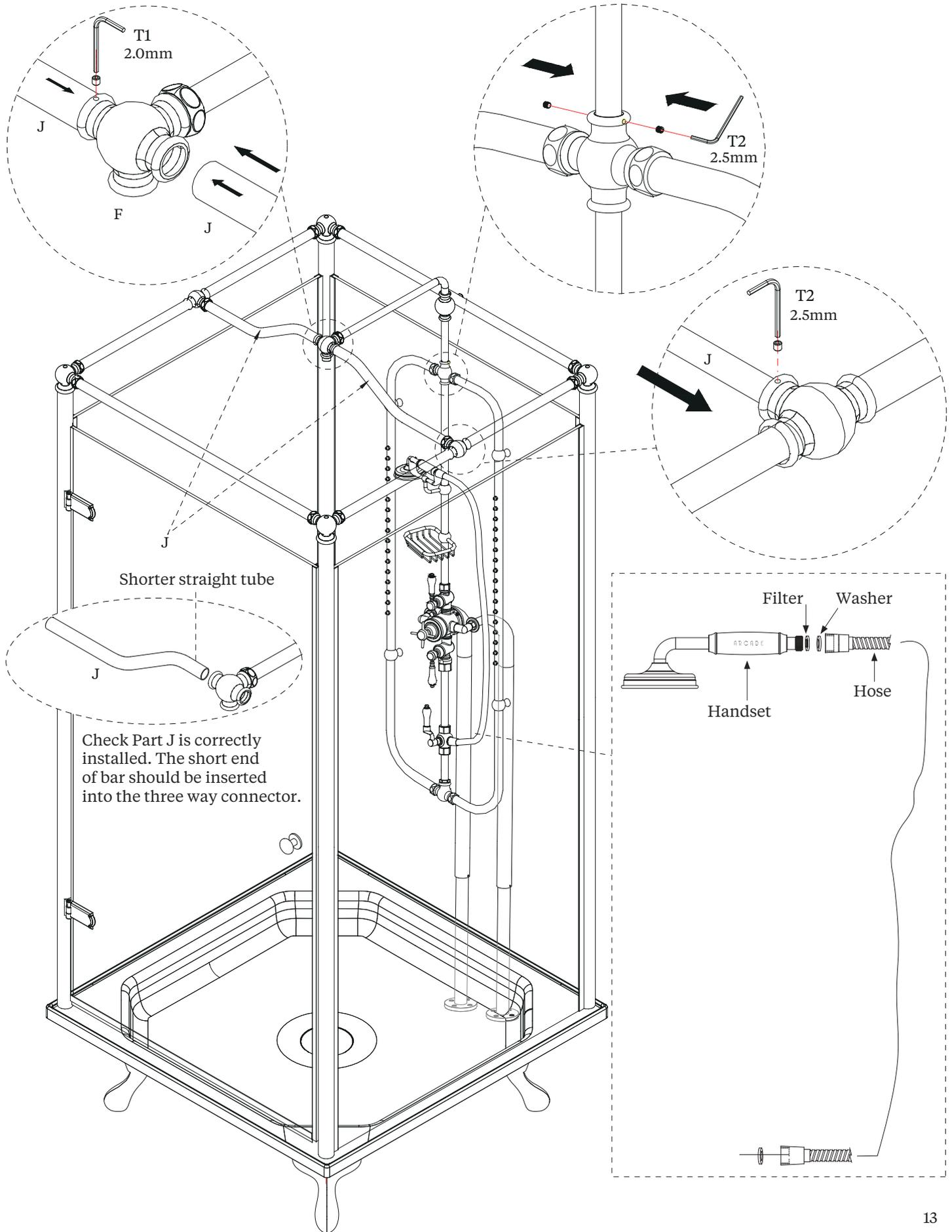
Check Part J is correctly installed. The short end of bar should be inserted into the three way connector.
