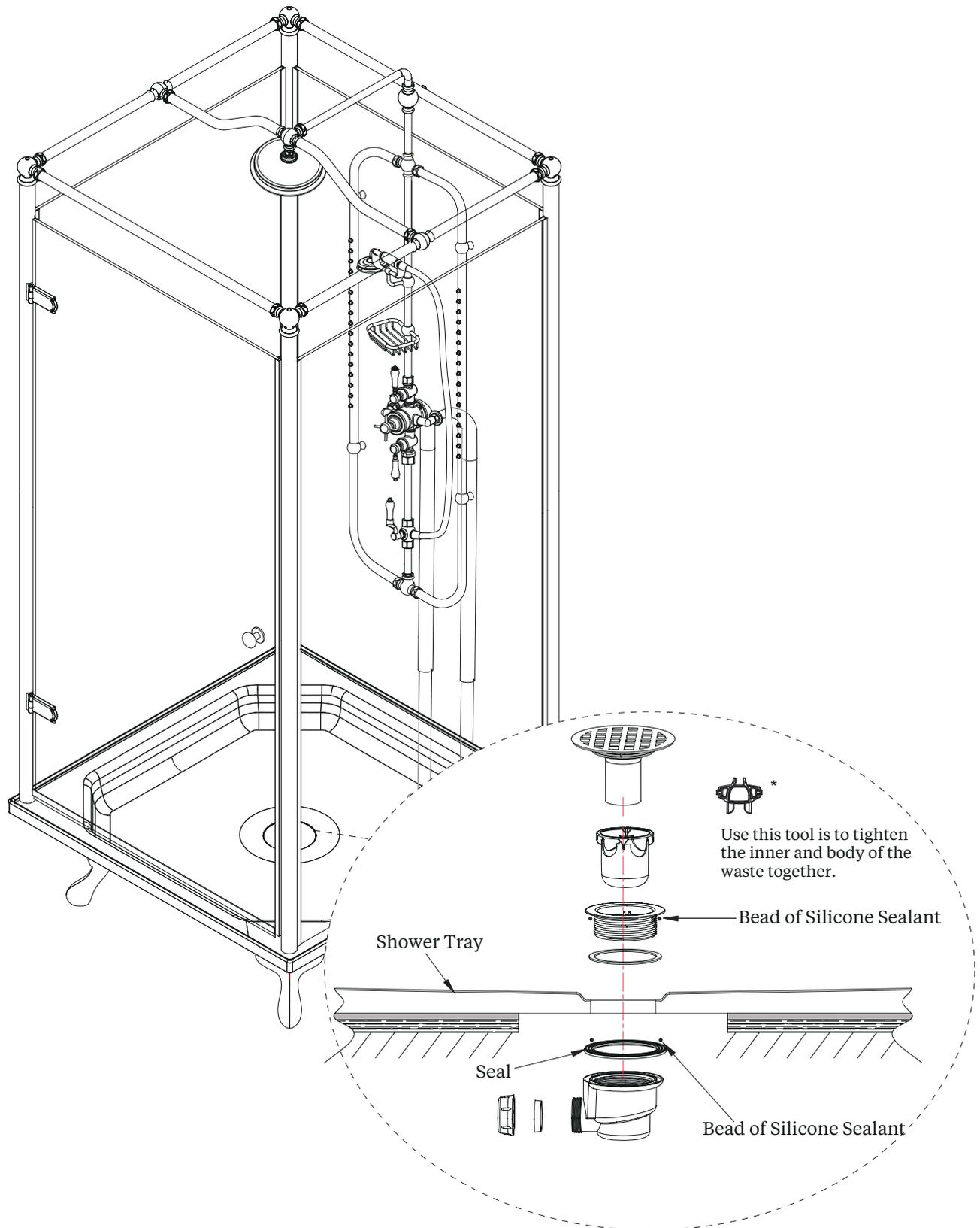
If needed, Arcade exposed trap ARCW21 NKL can be used to connect with the tray waste.
