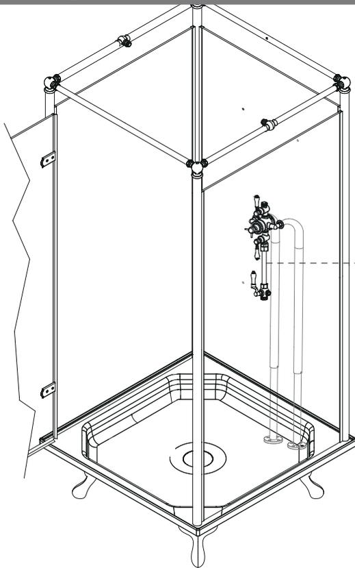
For a correct installation, the diverter handle should point upwards and face to the right.
