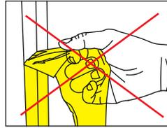
To protect the plating finish, yellow protective film has been placed on the profiles. The film should not be removed until installation is complete.
