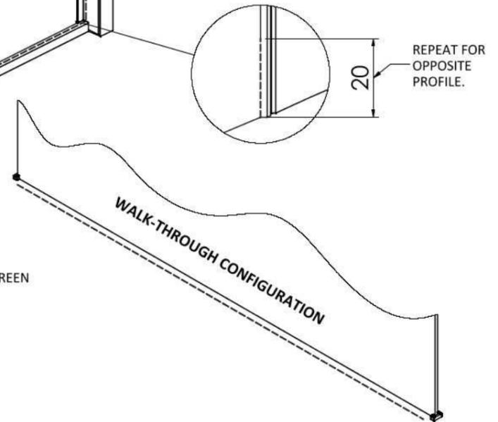
SILICONE SEAL ALONG THE OUTSIDE EDGE OF THE SCREEN WHERE THE GLASS MEETS THE TRAY/FLOOR IN A CONTINUOUS BEAD.
