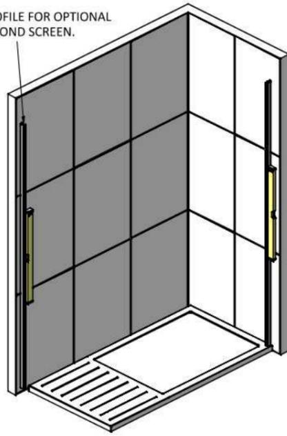
POSITION THE WALL PROFILES ON THE TRAY IN A SUITABLE POSITION. MAKE SURE THEY'RE TRUE WITH A SPIRIT LEVEL, THEN MARK THROUGH THE FIXING HOLES WITH A PENCIL. REMOVE PROFILES THEN DRILL AND PLUG THE WALL (ITEM 12). NOW FIX THE WALL PROFILE IN PLACE USING ITEM 11.
