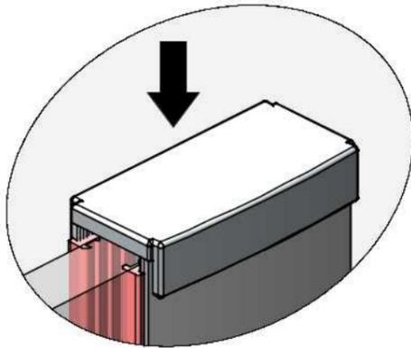
FIT THE WALL PROFILE CAP(S) (ITEM 4). A SMALL BLOB OF SILICONE CAN BE APPLIED TO THE UNDERSIDE OF THE CAP TO HOLD IT IN PLACE IF NECESSARY.
