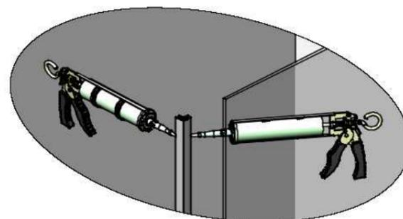
TO FIX THE OPTIONAL RETURN GLASS PANEL, FIRSTLY RUN A SMALL BEAD OF SILICONE DOWN THE INSIDE OF EACH GLASS SLOT IN THE CORNER PROFILE (ITEM 15) STOPPING 5mm SHORT AT EITHER END.
