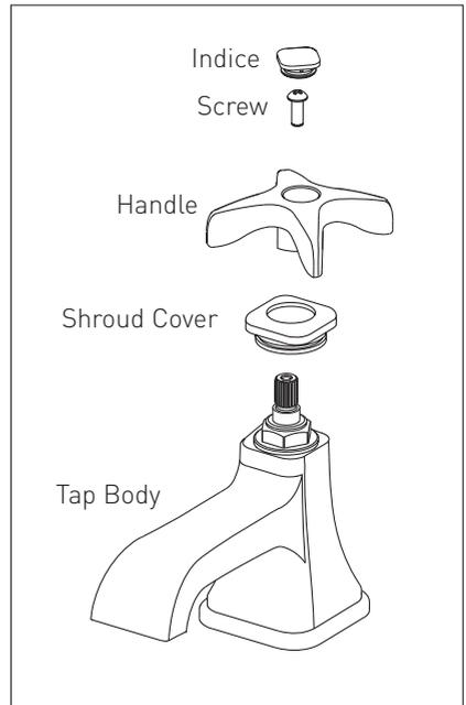
**⚠ Important:** Tighten the valve with the correct size socket and apply appropriate force/torque.
