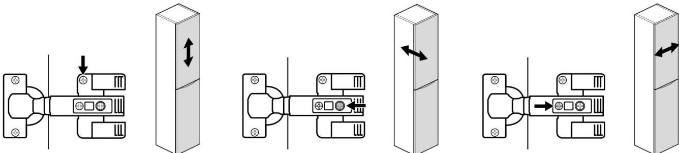
**To move door up or down:** Turn screw shown to move door up or down to suit
