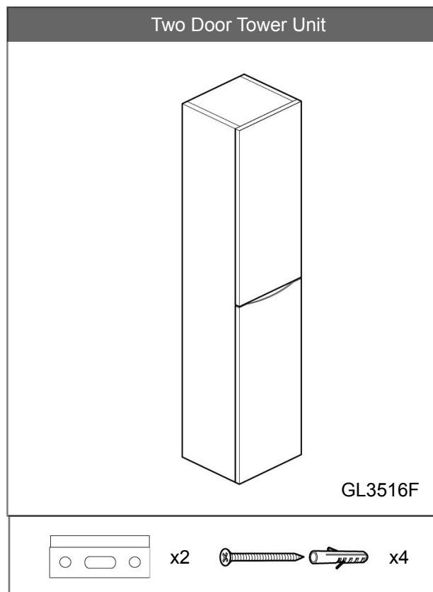
Tools & equipment needed: Drill, 8mm Suitable drill bit, Phillips screwdriver, Spirit level, Ruler/tape measure, Pencil, Silicone sealant (clear).
