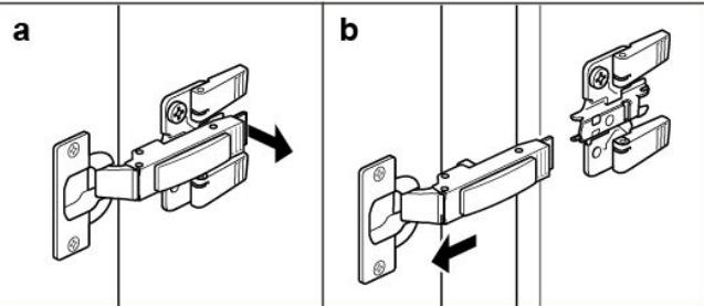
Remove the TOP door before installation. a: Lift the tab (shown) on both hinges, to release. b: Pull door back.
