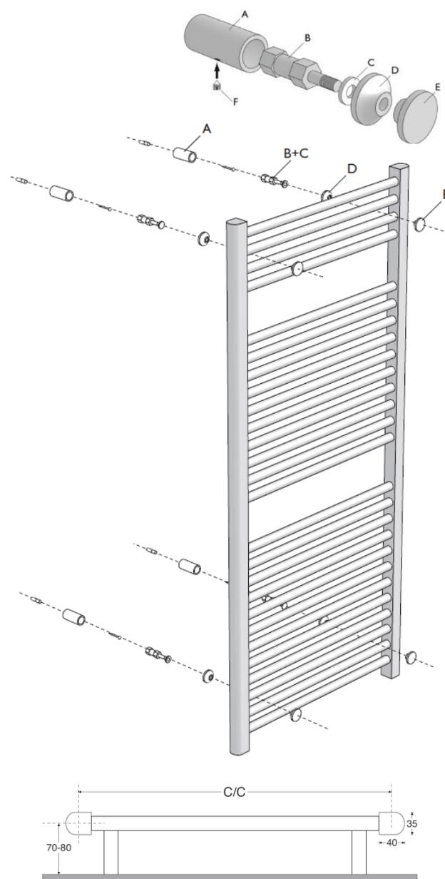
Tapping centres (C/C) for Hugo2 radiators are 40mm less than the width of the rail and 70mm out from the wall
