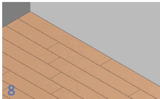
Remove the shims when you have laid all of the floor. The expansion gap is for when the floor expands if it is particularly hot or sunny.
