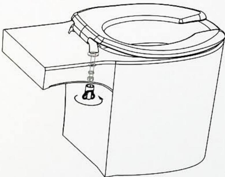
1. Slide the spacer washers onto the hinge lugs so that the threads are level with the holes on the pan.
