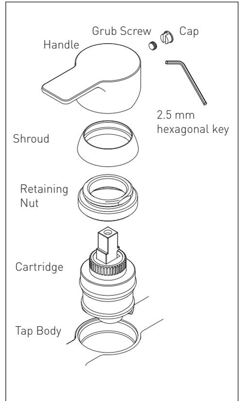
**!** **Important:** Tighten the retaining nut with the correct size spanner and apply appropriate force/torque. **Do not overtighten.**
