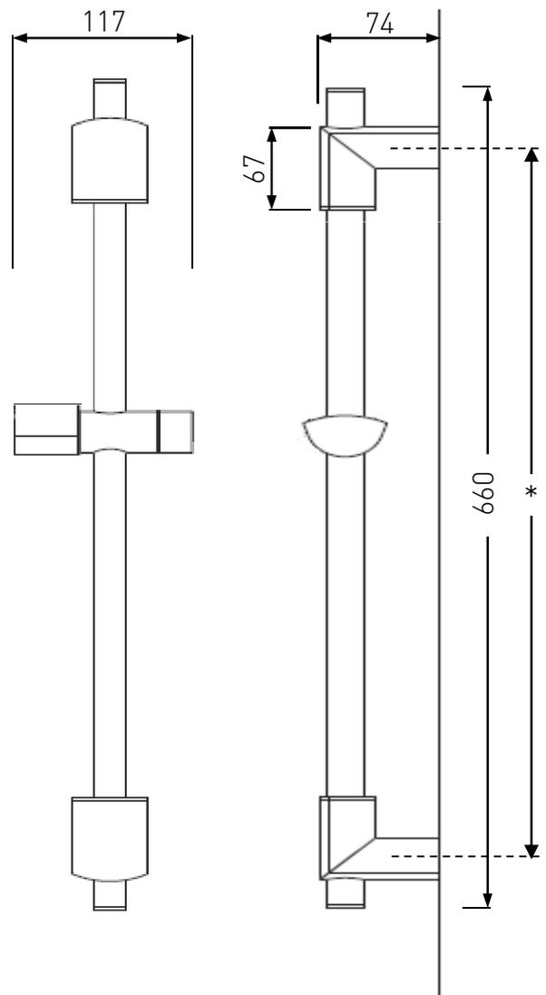
\* Note: The Riser rail wall brackets can be positioned up or down the riser rail as required. This allows any existing holes to be reused or covered by the wall brackets. The brackets can also be adjusted to sit in the middle of the tiles or in the tile joints.
