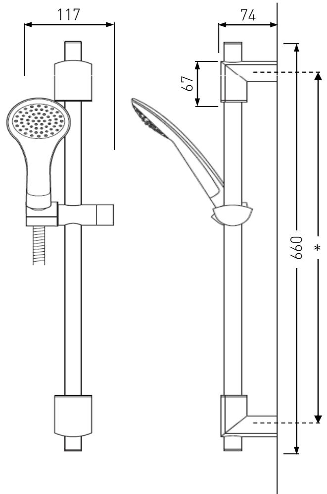
\* Note: The Riser rail wall brackets can be positioned up or down the riser rail as required. This allows any existing holes to be reused or covered by the wall brackets. The brackets can also be adjusted to sit in the middle of the tiles or in the tile joints.
