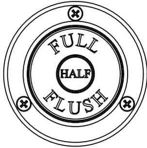
1. The push button can be positioned either Left or Right. Using a hole saw, cut a 38mm diameter hole into the surface you want the button (Fig 1 shows push button on the right).
