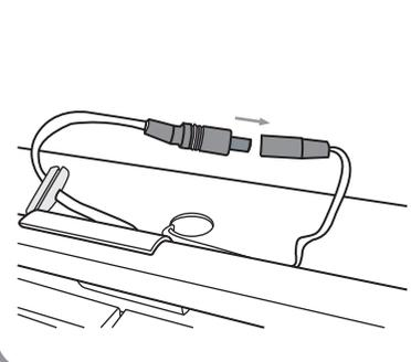
Push the connection and wires into the large hole on top of the cabinet. Place the rubber seal into the hole to hold the wire in place.
