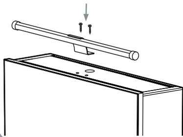
Plug the light fitting into the cabinet as shown.
