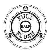
1. The push button can be positioned either Left or Right. Using a hole saw, cut a 38mm diameter hole into the surface you want the button (Fig 1 shows push button on the right).
