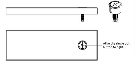
3. Remove the spacer block from the push button, this is not required.
