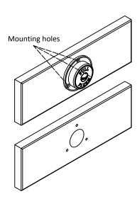
6. Attach the button using appropriate screws for the base material.
