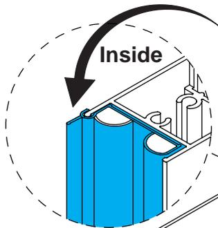
Ensure that the fixed panel with waterproof strip is positioned for assembly, so that the lip of the waterproof strip is going to be on the inside of the bath.
