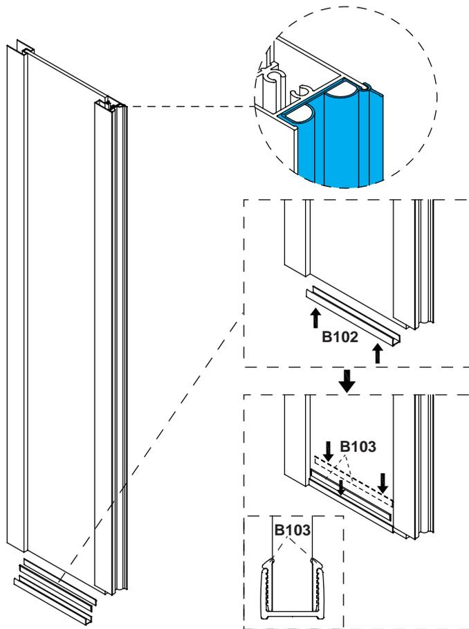
Ensure that the fixed panel with waterproof strip is positioned for assembly, so that the lip of the waterproof strip is going to be on the inside of the bath.
