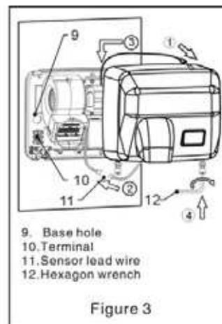
1. Remove the cover in order of ④③②① as shown in (Figure3); Do not overexert while removing the cover to prevent from breaking the wire between the cover and the base;
