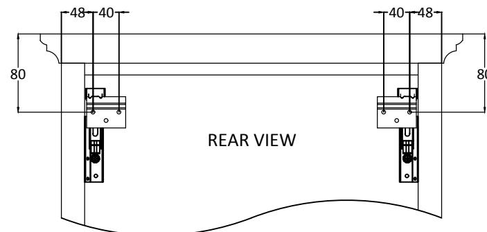
2. You may need to increase the hooks protrusion. To do this turn screw 'A' anti-clockwise. Once located onto the wall hanging plates, turn screw 'A' clockwise to fix the cabinet to the wall.
