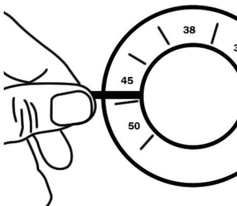
Using a 2.5mm Allen key, insert this into the hole where the chrome cap was fitted and loosen the grub screw about 1 turn to loosen.
