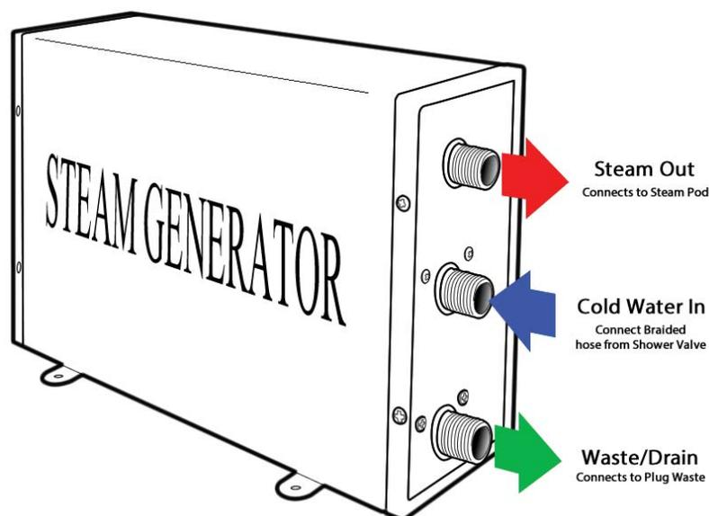
Cold Water IN from the shower valve connects to the Steam Generator (your steam generator may look different than the image opposite, but the connections are marked the same).
