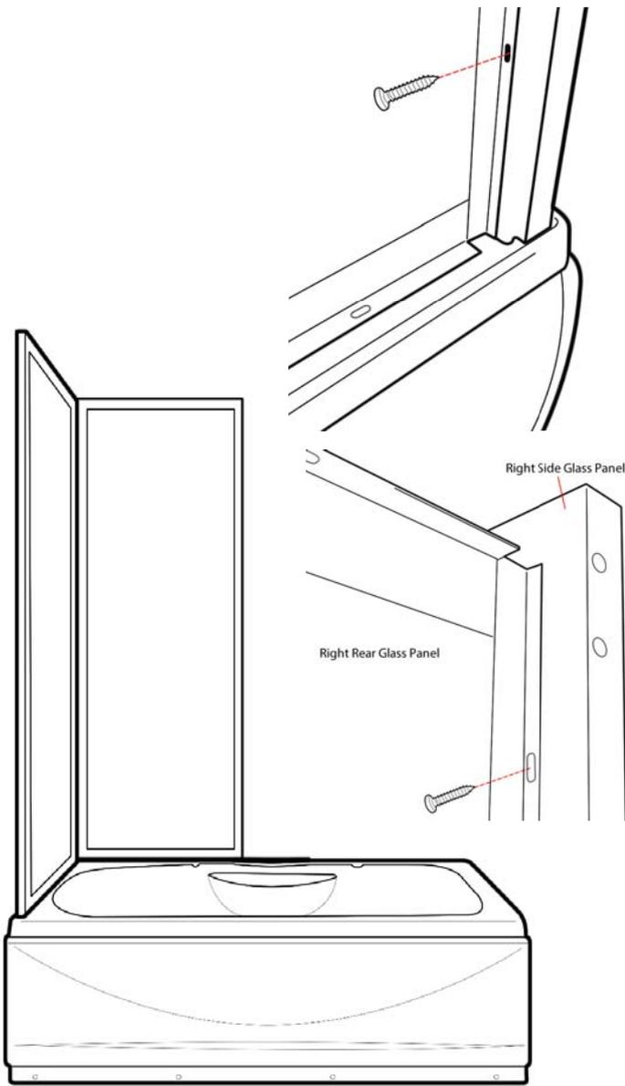
Now position the right hand side panels and repeat the process until the two rear panels and side panels are in position and fixed.
