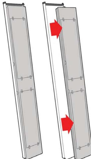
Fitted to the rear of the tower panel is a white plastic protective cover. This part is fitted to protect the valve and pipes during transport.
