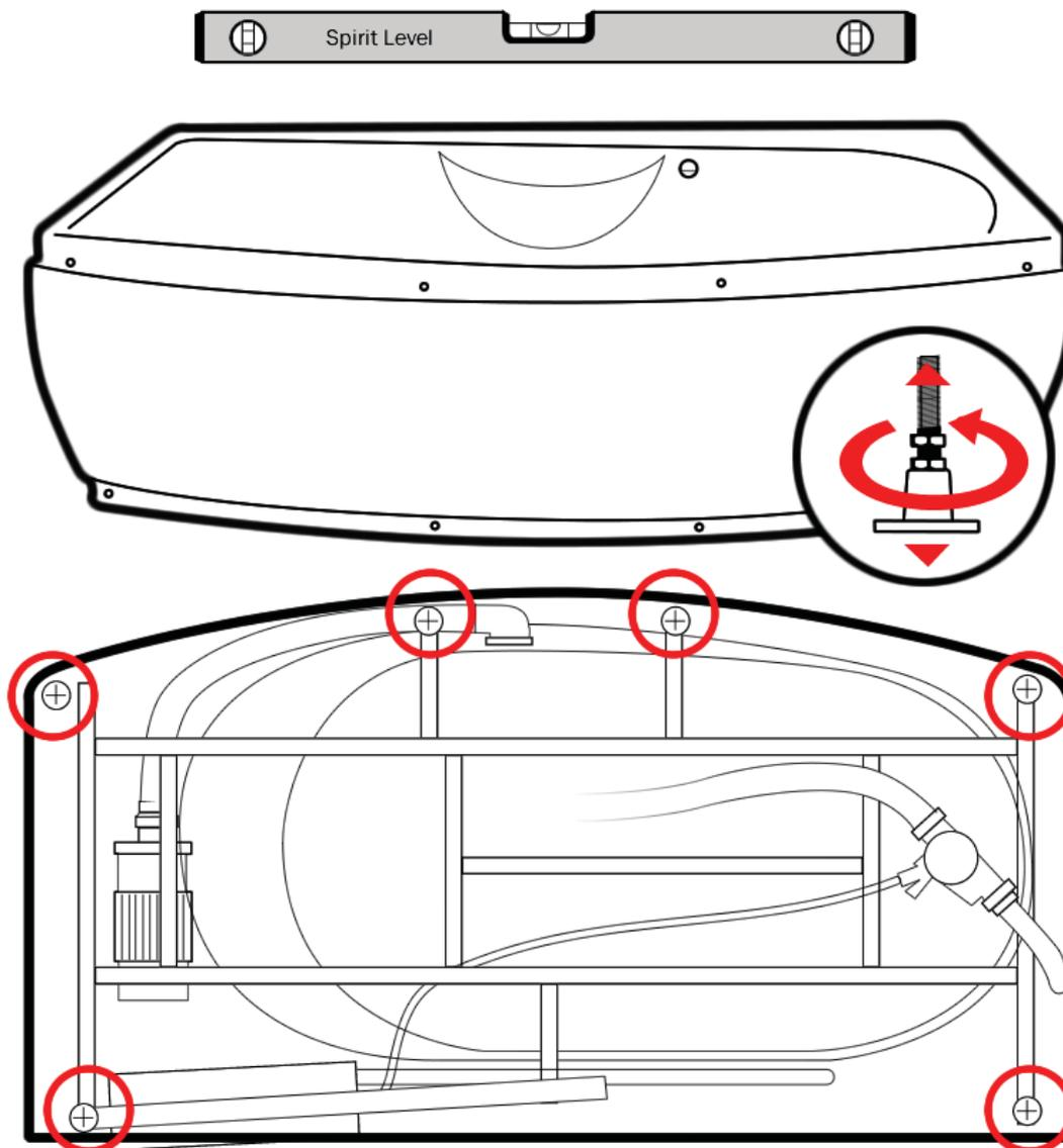
Position the tub base in what will be its final location and adjust the feet until the base is level. You can raise/lower the feet under the tub and with a spirit level laid across the tub, ensure the tub is level.
