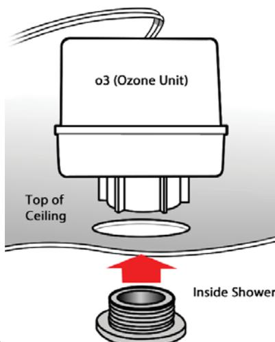
Unscrew the silver end and offer this on the inside aspect of the ceiling and screw this into the main body of the unit as it is placed on the upper side of the ceiling.
