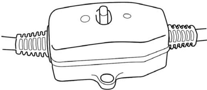
If the Main Board (Consumer Unit) in the property is already RCD protected you **MUST** remove the one fitted to this product.
