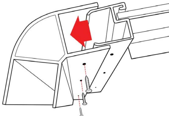
Diagram above shows the front right hand cover and frame with the screws to fix together.
