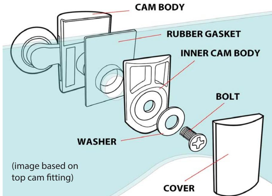
To fit each of the cams, first select the appropriate cam for the position on the door:
