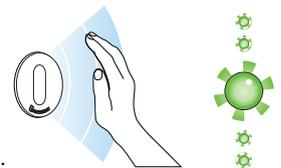
**C** When the water has run for the desired flush time, move your hand out of the line of sight of the sensor. The water will cease and the flush time will be set. It is recommended that this be set to a time that allows the trap to be refilled.
