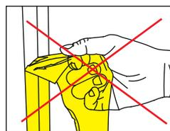
Yellow protective plastic film has been placed on the metal profiles. This film should not be removed until installation is complete. This is to protect the plating finish and prevent profiles being scratched during fitting. A pair of gloves are also provided to wear during installation, this will reduce oils and silicon stains being transferred during installation.
