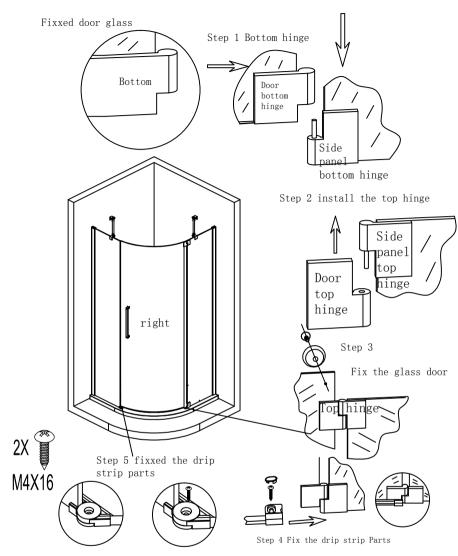
Step 1 Fit bottom hinge strap to the door(if not already fitted),slot the door bottom hinge strap onto the side panel bottom hinge strap. Step 2 solt the top door hinges strap onto the side panel top hinge strap Step 3 fix the glass door into the door top hinge strap and secure using the screws and caps provided.
