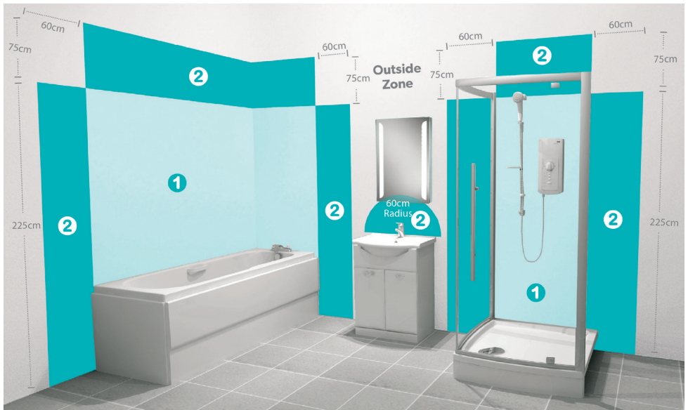
This product is IP21 - suitable for installation in zones: 2 & Outside Zone (Fig 4)
