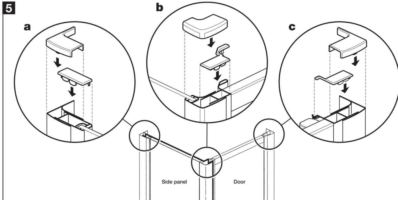
Push-fit the top caps onto the wall channels and corner post.
