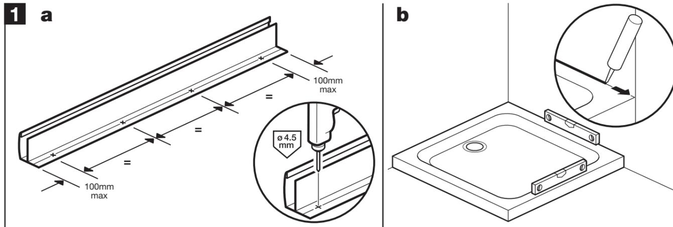
**a:** Drill holes in both wall channels at points shown using a 4.5mm drill bit, where shown.
