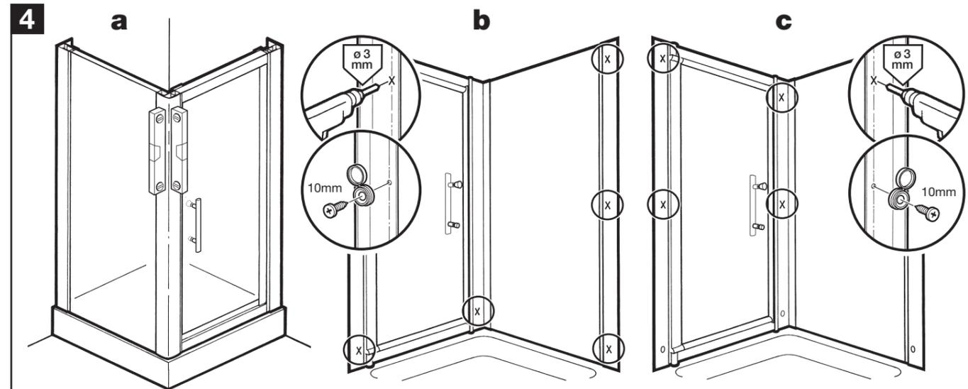
**a:** Check that the enclosure is perfectly vertical and the door is square within the frame (see Door instruction).
