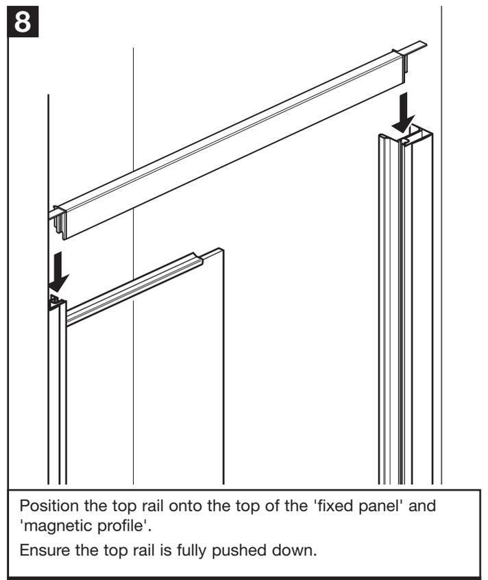
Position the top rail onto the top of the 'fixed panel' and 'magnetic profile'.
