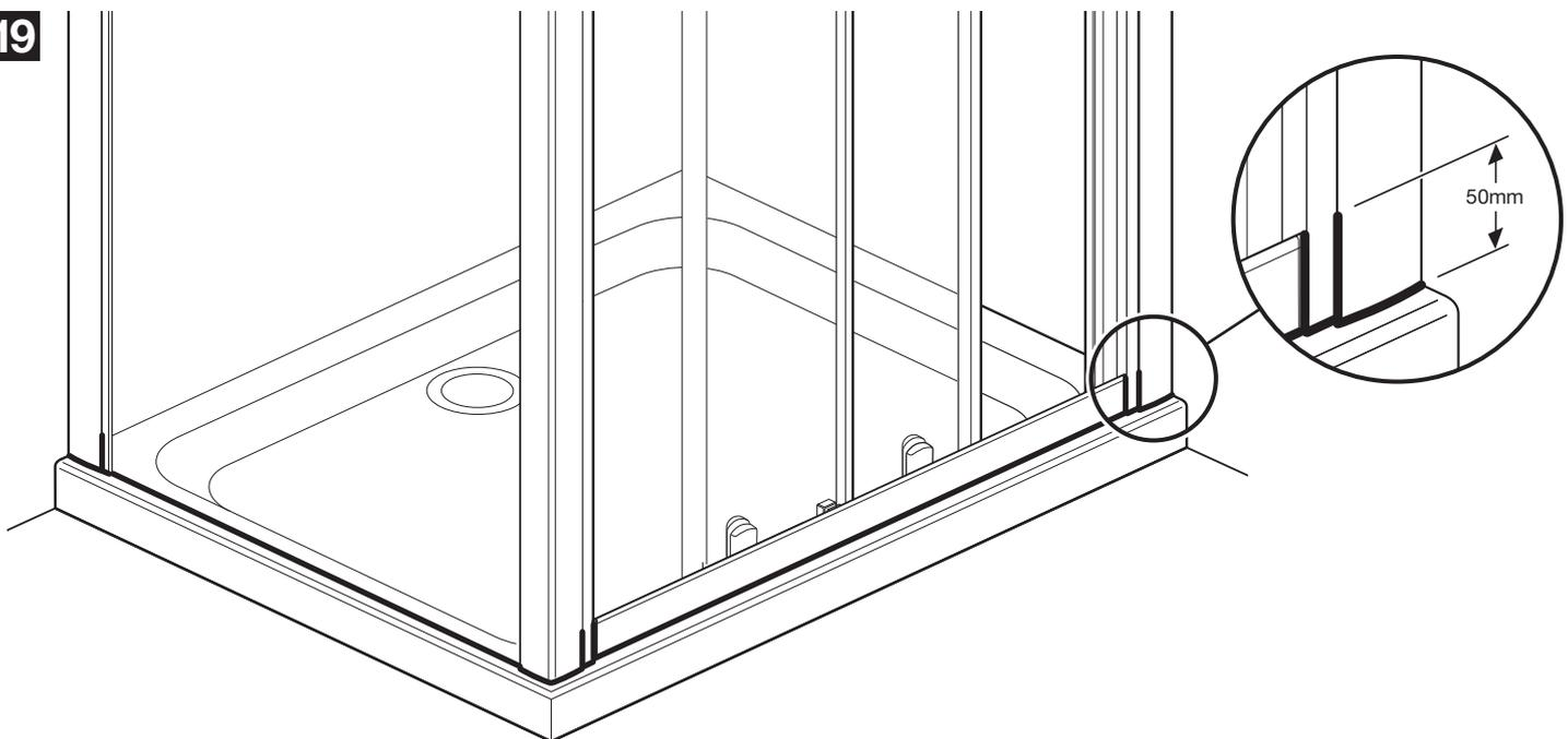
**From the outside only**, apply sealant to the bottom of the enclosure and 50mm up the wall channels and vertical joints as shown.
