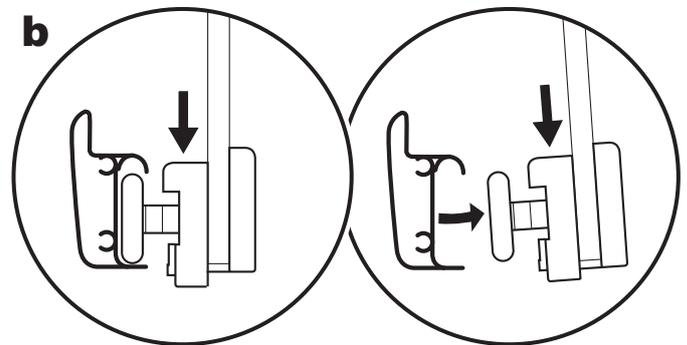
**Door adjustment:** The wheels at the top of the door may need adjusting so that the door slides freely and the magnetic seal meets evenly with the magnetic profile when the door is closed.
