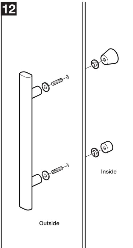
Fit the door handle (PN60510) to the door ensuring the washers fit between the glass and handle.
