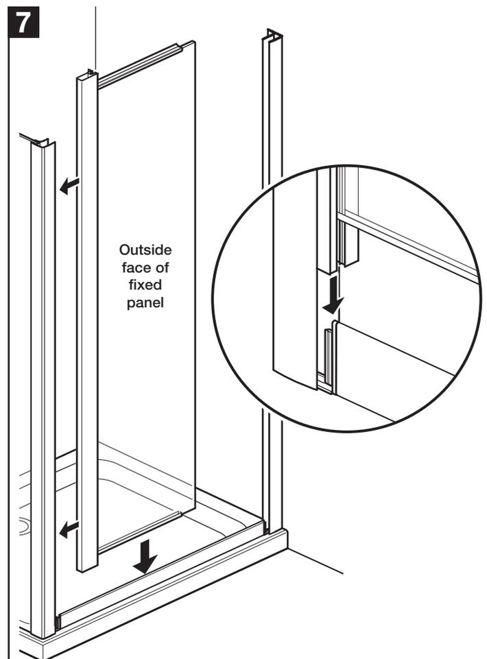
Position the fixed panel into the required corner post/wall channel and slide down so it fully slots onto the end moulding of the bottom rail.
