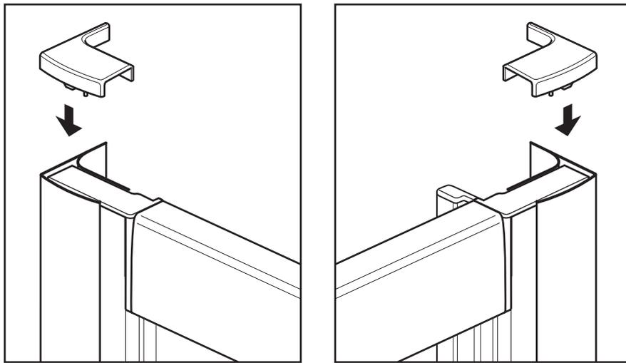
Push fit the top caps (PN50493/50494) onto the wall channels as shown
