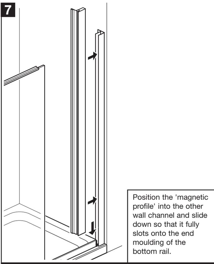
Position the 'magnetic profile' into the other wall channel and slide down so that it fully slots onto the end moulding of the bottom rail.
