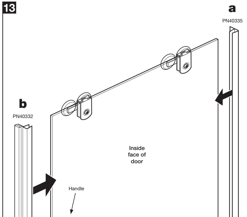
**a:** Select vertical seal (PN40335) with the 20mm 'flipper' and fit onto the back edge of the door. **Ensure the flipper seal 'flap' is on the outside of the door.**
