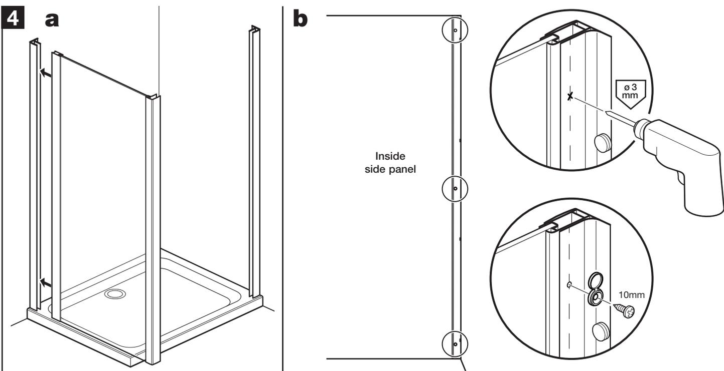
**a:** Insert the side panel into the wall channel ensuring that the corner post is the same distance in from the edges of the tray as the wall channels.
