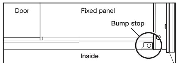
The enclosure can be assembled with the side panel on either the right or left and the door on either the right or left (see step 5). **Note:** The bottom bump stop **MUST** be on the 'fixed panel' side of the enclosure.
