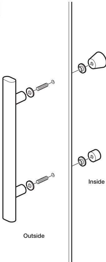
Fit the door handle (PN60510) to the door ensuring the washers fit between the glass and handle.
