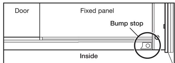
The enclosure can be assembled with the side panel on either the right or left and the door on either the right or left (see step 5). **Note:** The bottom bump stop **MUST** be on the 'fixed panel' side of the enclosure.
