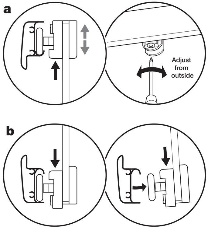
**Door adjustment:** The wheels at the top of the door may need adjusting so that the door slides freely and the magnetic seal meets evenly with the magnetic profile when the door is closed.
