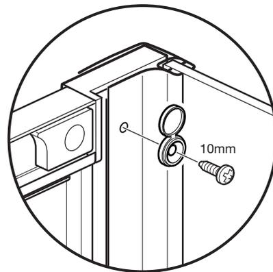
Check the door frame is vertical and is centrally positioned between the corner post and wall channel.
