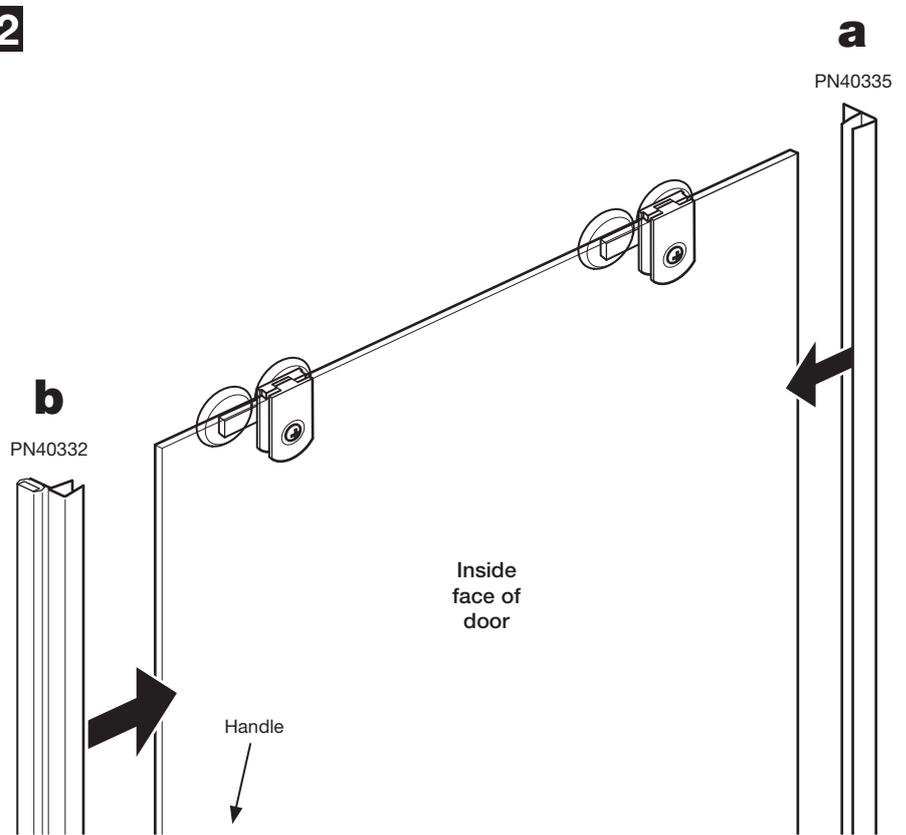
**a:** Select vertical seal (PN40335) with the 20mm 'flipper' and fit onto the back edge of the door. **Ensure the flipper seal 'flap' is on the outside of the door.**
