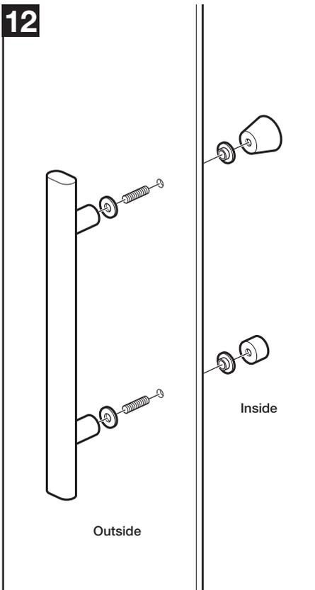
Fit the door handle (PN60510) to the door ensuring the washers fit between the glass and handle.
