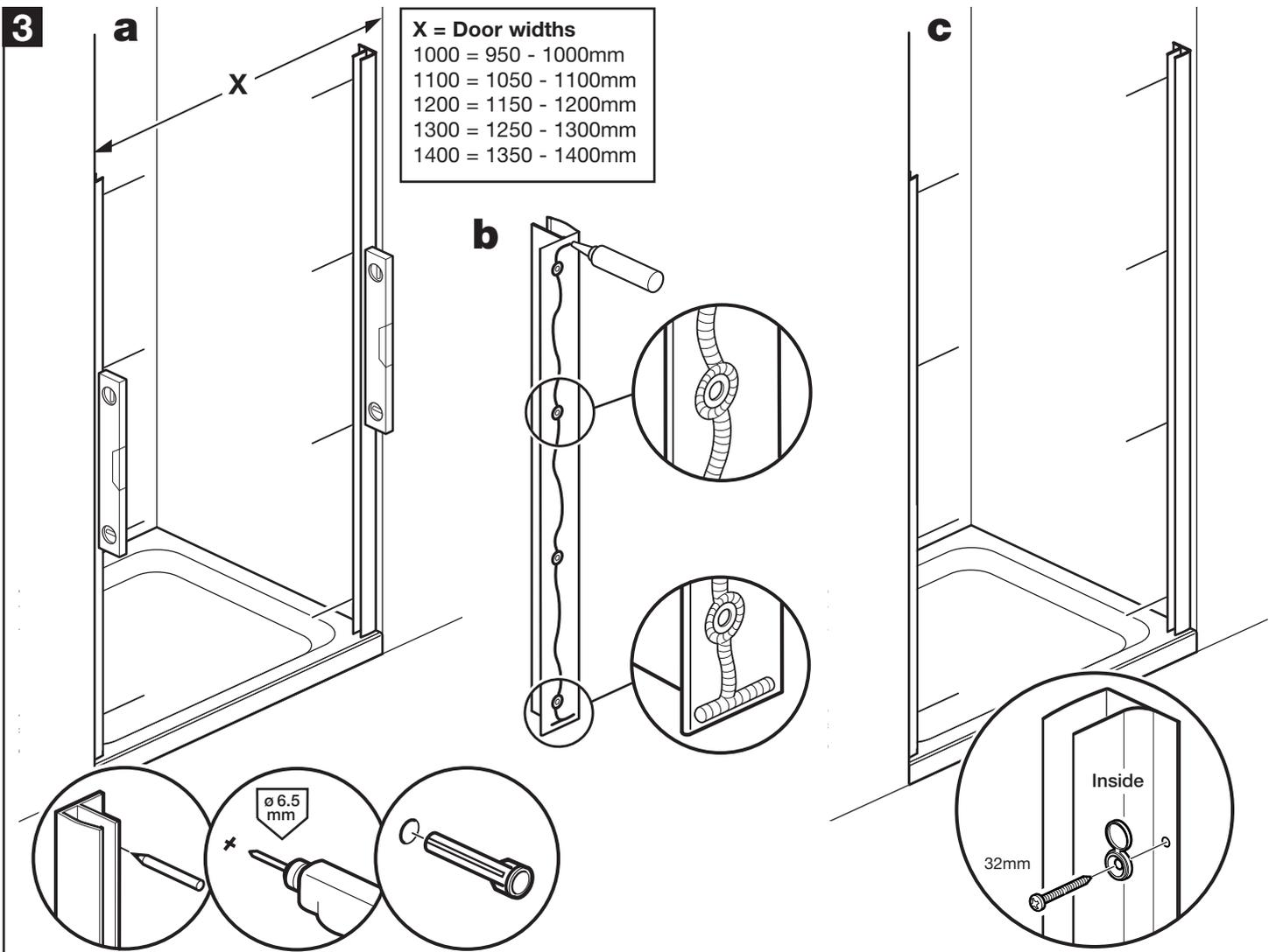
**a:** Place the wall channels on the tray ensuring they are vertical and an equal distance back from the front of the tray. Place masking tape against the wall before marking drill hole positions, this will help prevent the drill bit slipping. Drill 6.5mm holes, 30mm deep and insert the wall plugs.
