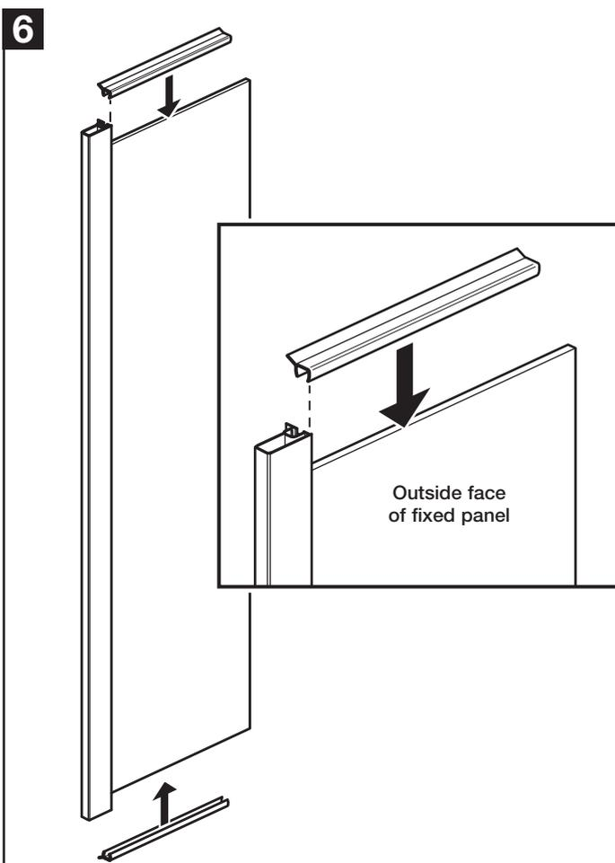
Push fit the 'short flipper seals' onto the top and bottom edges of the fixed panel - flush against the metal profile.
