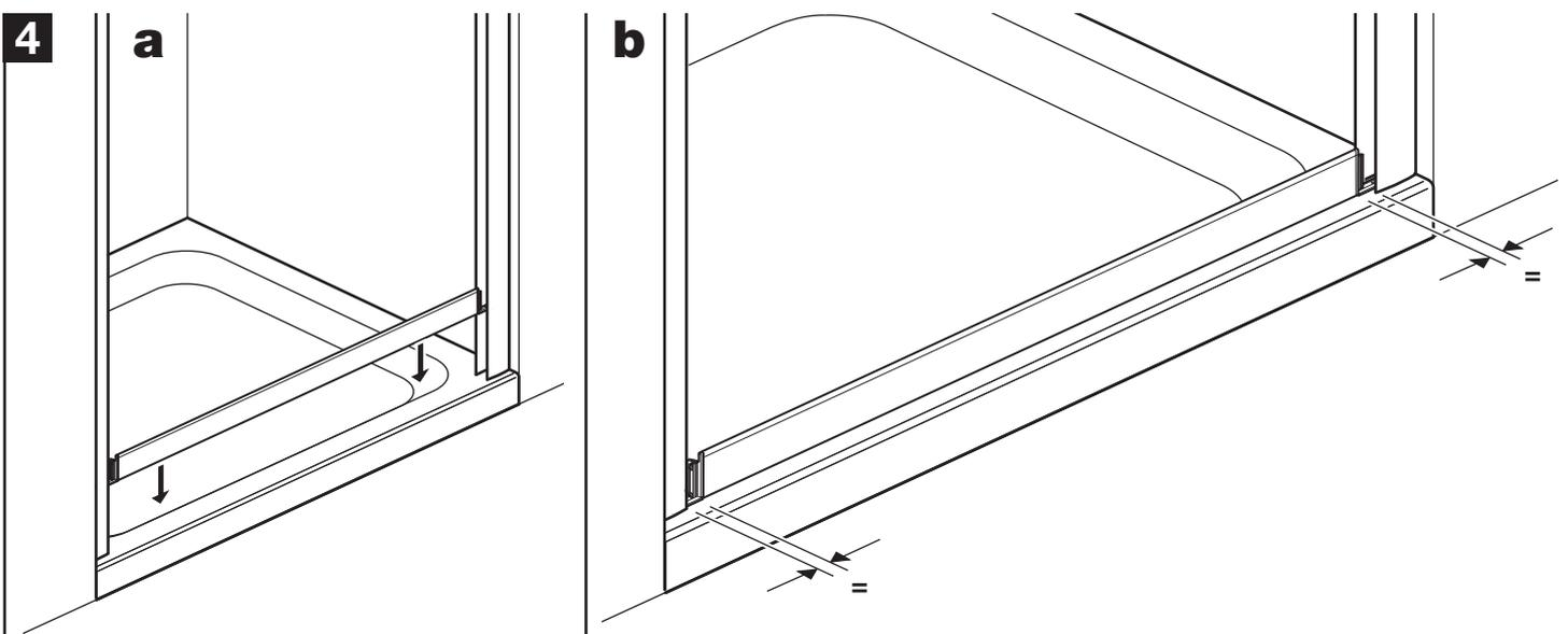
**a:** Place the bottom rail onto the tray with its end mouldings inserted into the wall channels.
