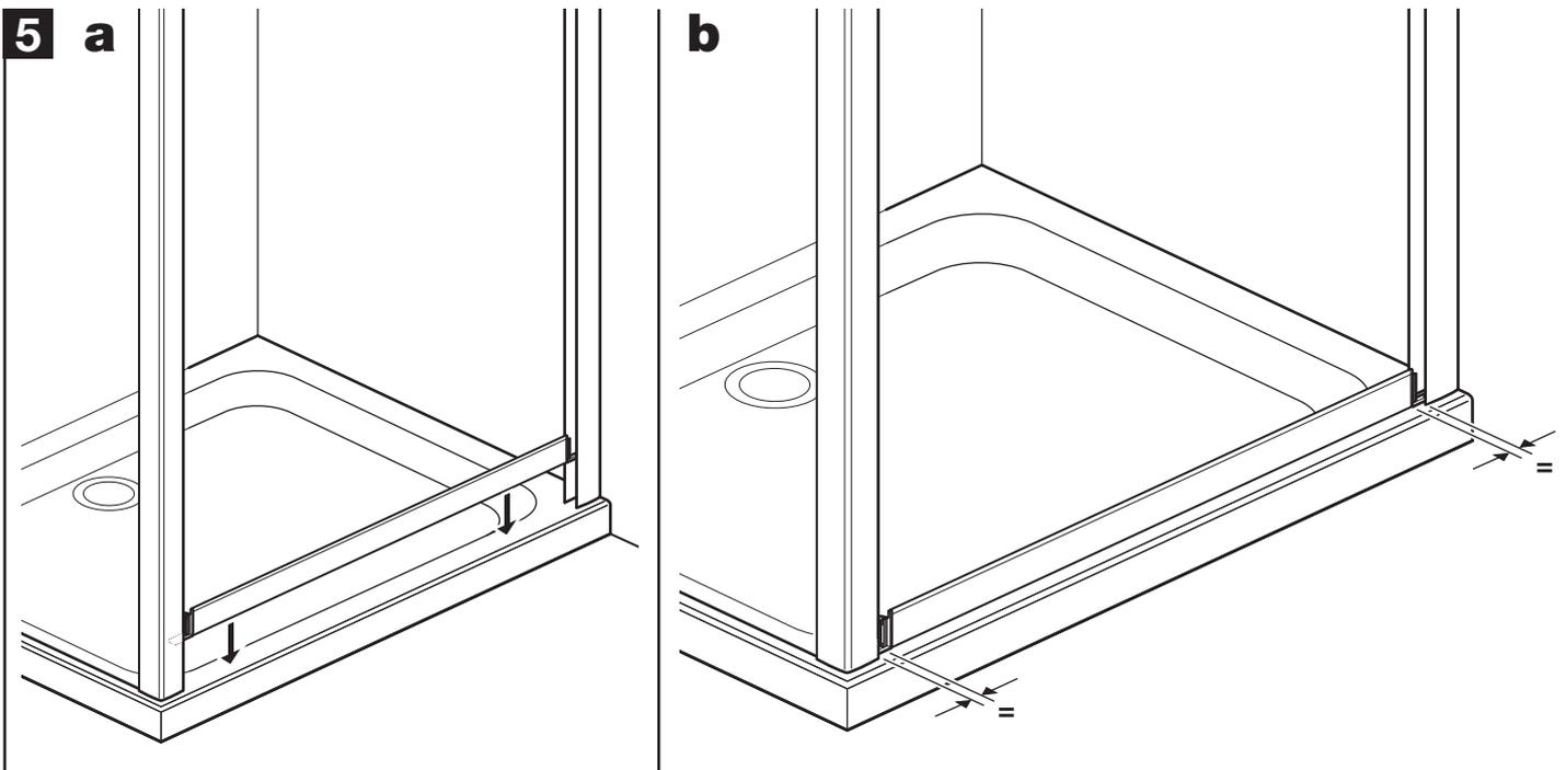
**a:** Place the bottom rail onto the tray with its end mouldings inserted into the corner post and wall channel.
