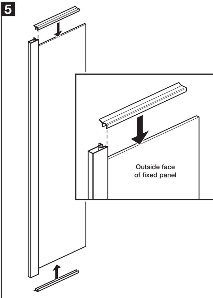
Push fit the 'short flipper seals' onto the top and bottom edges of the fixed panel - flush against the metal profile. **Ensure the flipper seal 'flaps' are on the inside of the fixed panel.**
