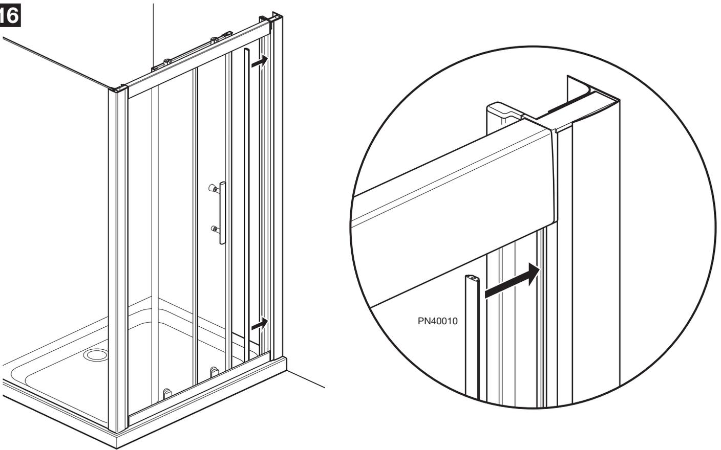
Push fit the seal (PN40010) into the 'magnetic channel profile'.
