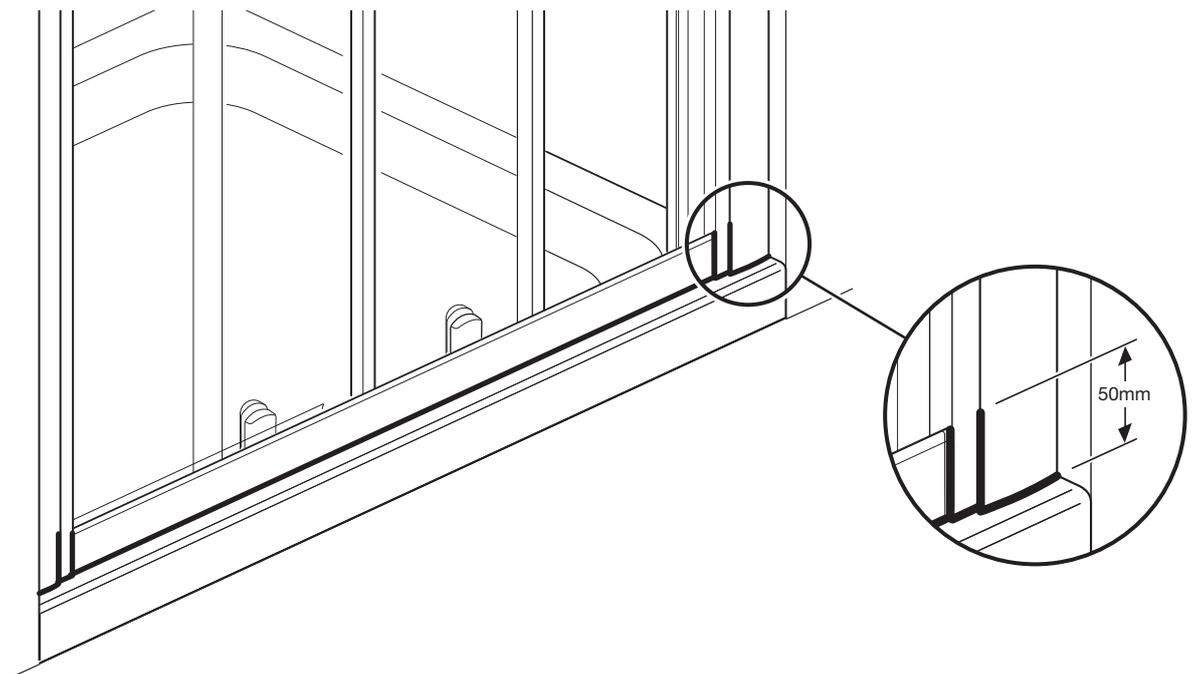
**From the outside only**, apply sealant to the bottom of the enclosure and 50mm up the wall channels and vertical joints as shown.
