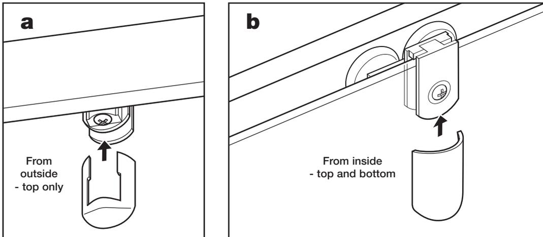
**a:** From outside the enclosure push fit the outer wheel covers onto the wheels at the top of the door.
