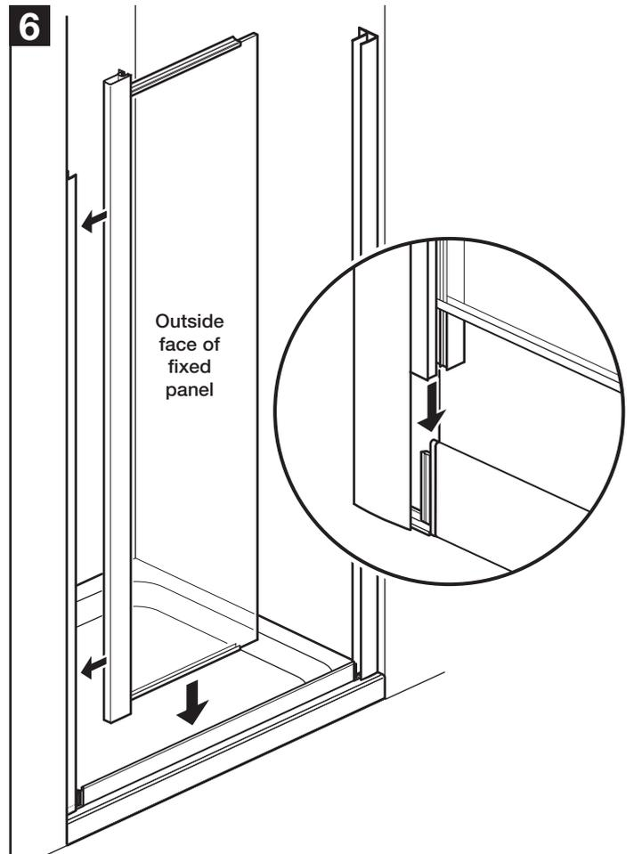
Position the fixed panel into the required wall channel and slide down so it fully slots onto the end moulding of the bottom rail.
