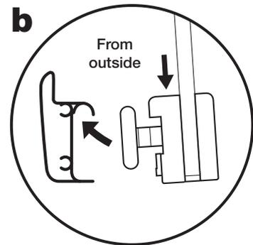
**a:** From inside the enclosure, position the top wheels into the top rail. **b:** From outside the enclosure with the door closed, push down the 'plungers' on both bottom wheels, position into the bottom rail and release.
