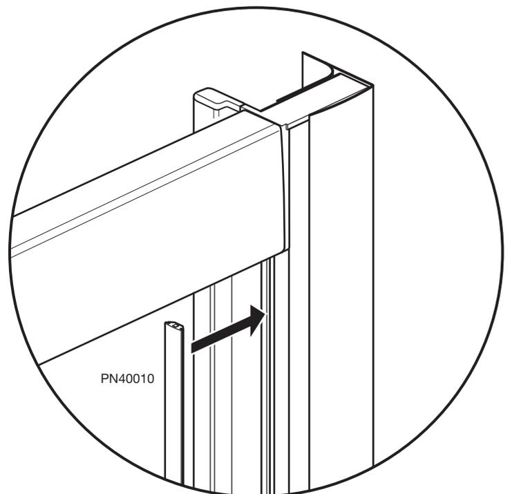
Push fit the seal (PN40010) into the 'magnetic channel profile'.
