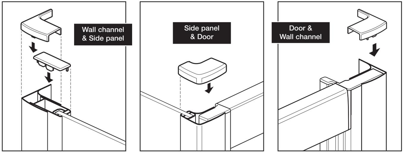
Push fit the top caps onto the wall channels and corner post as shown.
