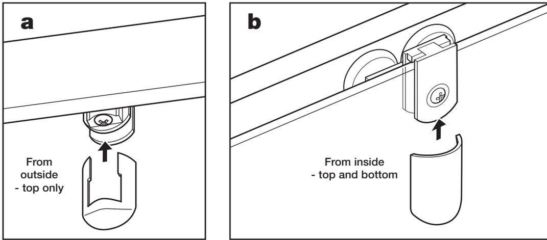
**a:** From outside the enclosure push fit the outer wheel covers onto the wheels at the top of the door.
