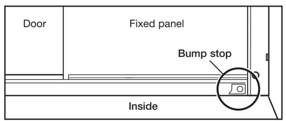
The enclosure can be assembled with the door on either the right or left side of the assembly (see step 4). **Note:** The bottom bump stop **MUST** be on the 'fixed panel' side of the enclosure.
