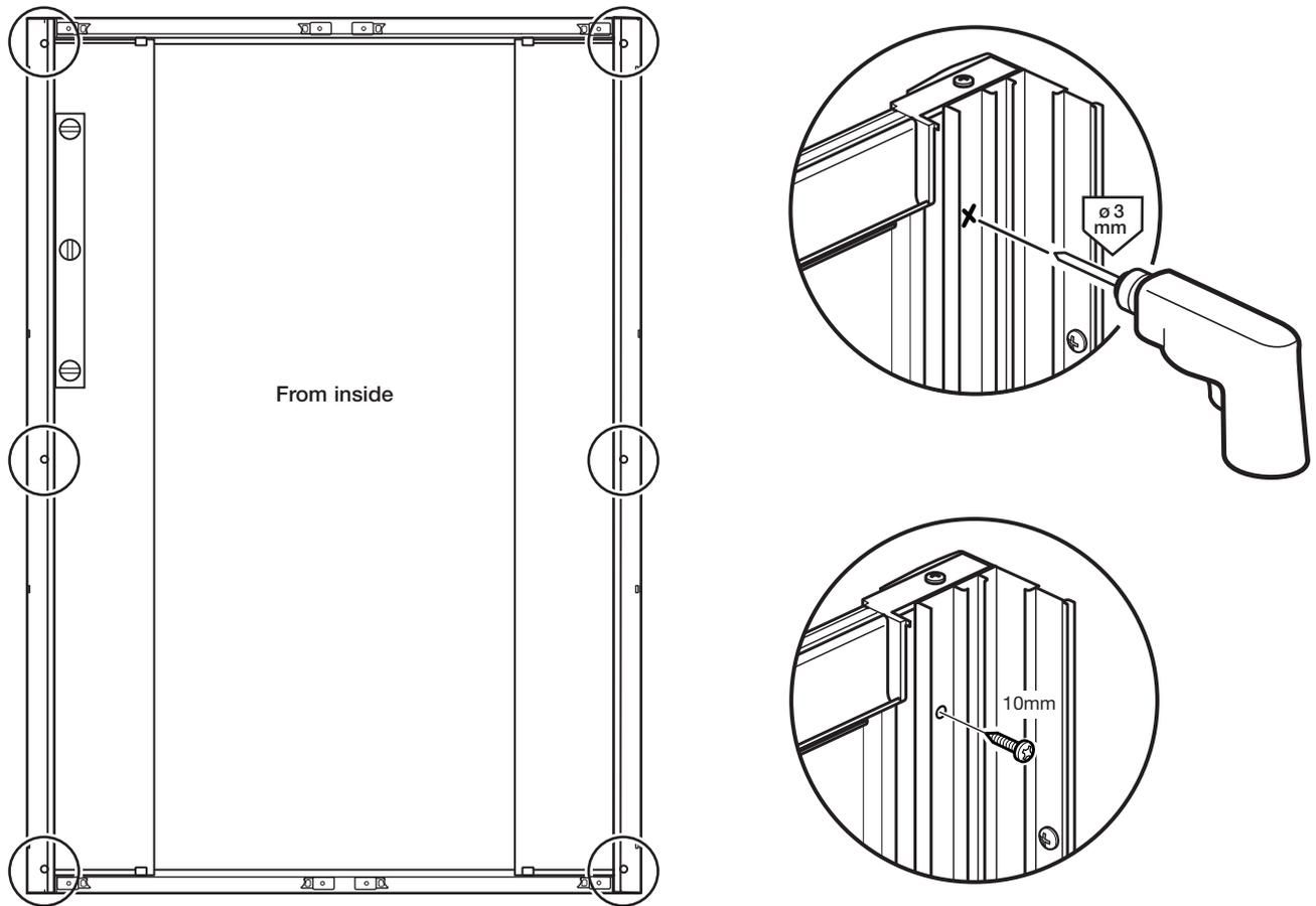
Check the door frame is vertical and is centrally positioned between the wall channels.
