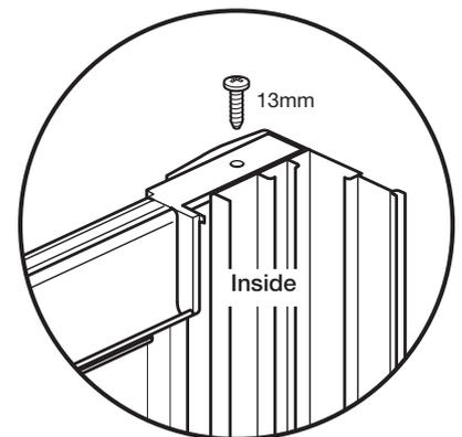
Position the top rail onto the top of the 'fixed panels'. Adjust the position of the fixed panel brackets as required.
