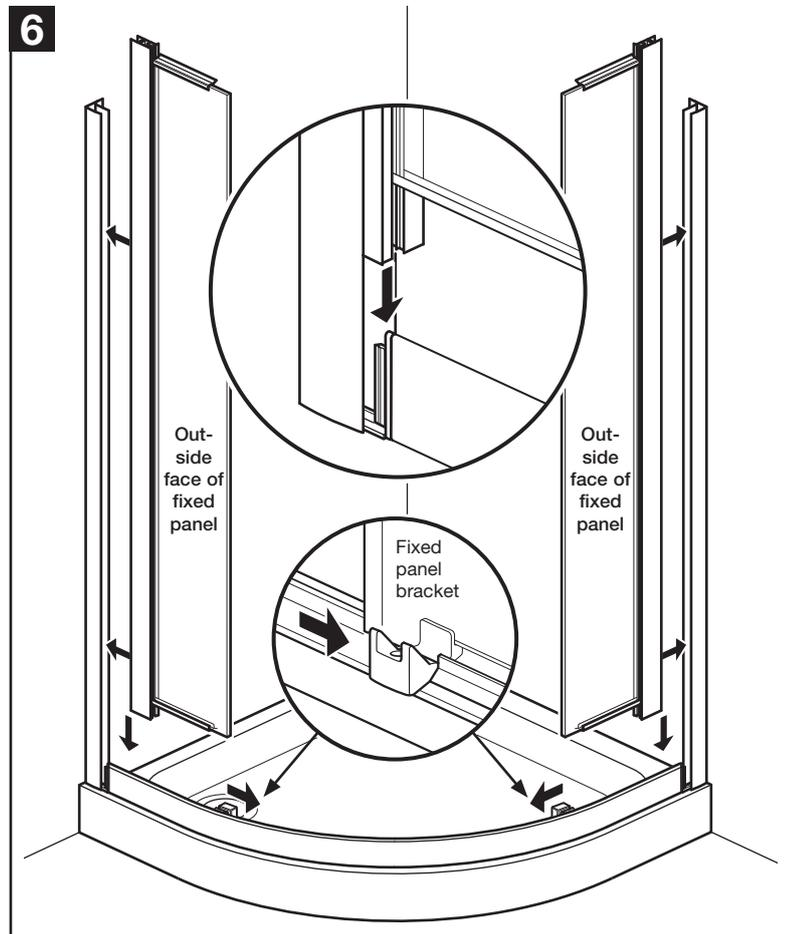
Position the fixed panels into the wall channels and slide down so that they fully slot onto the end mouldings of the bottom rail. Inside the enclosure, ensure the panels sit in the 'fixed panel brackets', slide the fixed panel brackets along the rails and position under the panels as shown.
