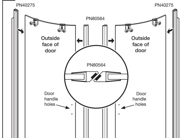
Push fit 'flipper seals' (PN40275) onto the back edge of the doors. **Ensure the flipper seal 'flaps' are on the outside of the doors.**
