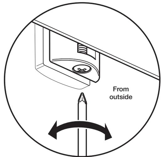
The 'wheels' at the top of the doors may need adjusting so that the doors slide freely and the magnetic seals meet evenly when the doors are closed.
