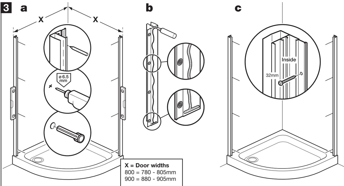
**a:** Place the wall channels on the tray ensuring they are vertical and an equal distance back from the front of the tray. Place masking tape against the wall before marking drill hole positions, this will help prevent the drill bit slipping. Drill 6.5mm holes, 30mm deep and insert the wall plugs. **b:** Apply sealant to the back of the wall channels and around the fixing holes. **c:** Fix the wall channels to the walls using 8 x 32mm screws.
