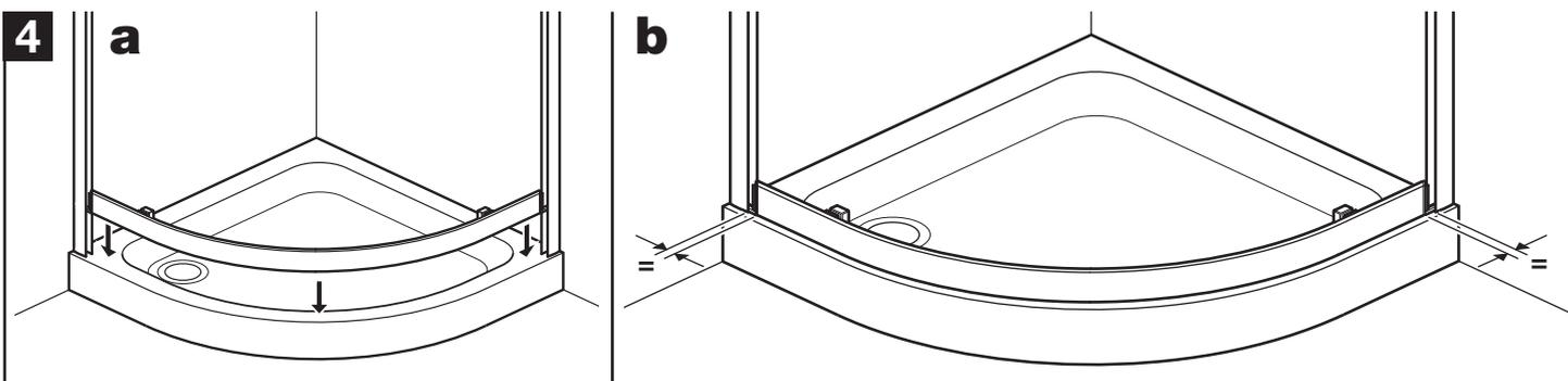
**a:** Place the bottom rail onto the tray with its end mouldings inserted into the wall channels.
