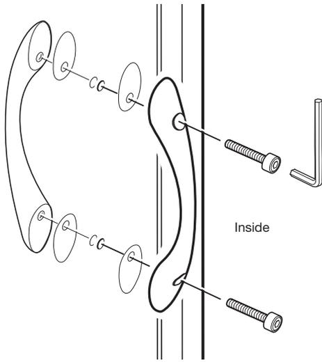
Fit the door handles to the doors with the allen bolts on the inside of the door.
