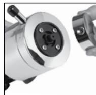
**5** Ensuring the black protective cap remains fitted, set the temperature control lever to the full cold (9 o'clock) position. Remove the fixing screws, pull the assembly clear and set aside.
