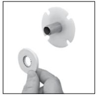
**3** Trim the projecting pipe to a length of 15-20mm, measured from the front face of the grip ring, using a rotary type cutter. If a hacksaw is used, the pipe end must be carefully de-burred and chamfered.
