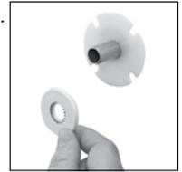
**3** Trim the projecting pipe to a length of 20-50mm, measured from the front face of the grip ring, using a rotary type cutter. If a hacksaw is used, the pipe end must be carefully de-burred and chamfered.
