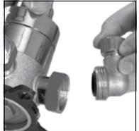
**!** The Siren concealed valve is supplied with an outlet cap at the bottom of the valve assembly allowing for a top outlet connection. If required the cap can be removed with a suitable tool and refitted to the top outlet of the valve.
