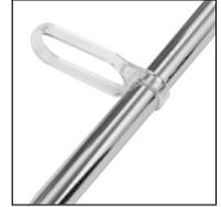
**14** Current water supply regulations state that the handset should not be allowed to pass a point 25mm above the spill over level of the bath or shower tray. If this cannot be achieved, the hose must be passed through the gel hook which has also been designed to be utilised as a hose restraint.
