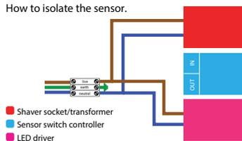
Re-wire the cabinet as shown in the diagram above. HiB recommends that all electrical bathroom products should only be fitted by a suitably qualified, Part P registered electrician.
