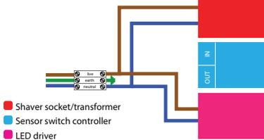
Rewire the cabinet as shown in the diagram above. HIB recommends that all electrical bathroom products should only be fitted by a suitably qualified, Part P registered electrician.
