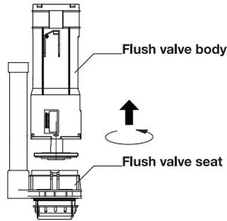
Install flush valve seat and seal as shown
