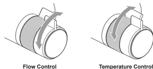
\* Reduced Flow Override - reduces water flow by up to 30% (dependant on inlet pressures) and can be overridden by increasing flow to full.
