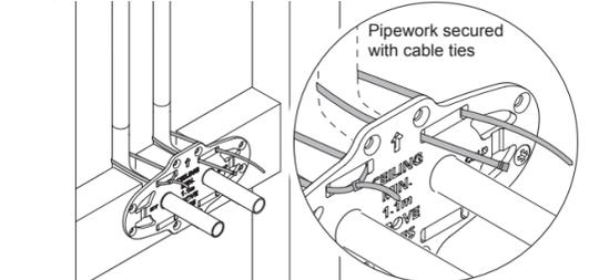
**Important!** Failure to secure the pipework may result in the pipework pushing back into the wall when fitting the mixer valve.
