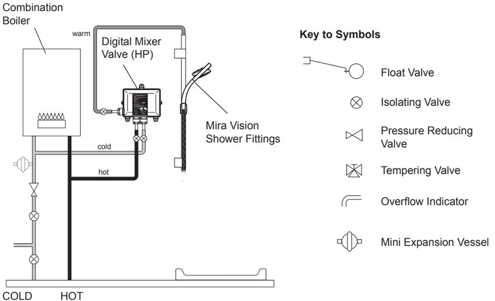
Only install the High Pressure Digital Mixer Valve with a multipoint gas water heater or combination boiler of a **fully modulating design** (i.e. where the water draw-off rate indirectly controls the gas flow rate to the burner).
