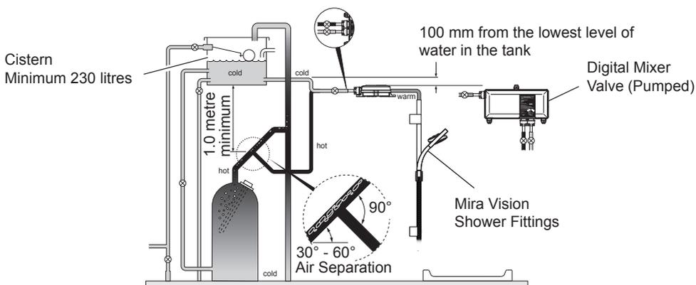
The shower control **must** be fed from a **cold water storage cistern** and a **hot water cylinder** providing nominally equal pressures. Pipework layouts and connections **must** be such that other draw-offs will not effect water supplies to the shower, shared supplies may lead to airlocking or water starvation. It is therefore best practice to have independent hot and cold supplies to the Low Pressure (pumped) Digital Mixer Valve.
