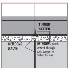
**Continue panelling:** Continue panelling around the room fixing each panel to the battens with Reef adhesive, and/or screws through the back lip of grooved edge. Seal tongue and groove joints using Reef sealant. Use internal and external corner profiles, sealing with Reef sealant, where appropriate.
