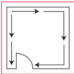
**Where to start:** Start at the corner furthest from the door, panel in both directions around the room. The last panel is fitted above the doorway, placed in position tongue first and swung into position. All panels must be correctly aligned and plumb, allowing for 3mm expansion gaps. Fix panels to battens using Reef panel adhesive. Seal all panel joints using Reef sealant.
