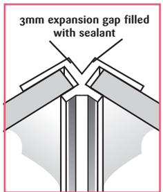
**Begin panelling:** First fix a Reef internal corner profile in position ensuring that it is plumb. Apply Reef sealant to the recess of the profile. Apply Reef adhesive to the battens. Insert the first panel after removing the smaller tongue, or cutting to size. Then continue to panel away from the corner in both directions, fixing panels to battens with Reef adhesive, and sealing joints with Reef sealant. Allow for 3-4mm expansion gaps, filled with Reef sealant.
