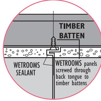
Vertical edges tongued and grooved giving finished panelling a smooth, easily maintained surface. Each panel has a symmetrical tongued and grooved vertical edges to give 5mm of joint overlap. When sealed with Reef sealant a waterproof joint is assured.
