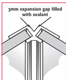
**Begin panelling:** First fix a Reef internal corner profile in position ensuring that it is plumb. Apply Reef sealant to the recess of the profile. Apply Reef adhesive to the battens. Insert the first panel after removing the smaller tongue, or cutting to size. Then continue to panel away from the corner in both directions, fixing panels to battens with Reef adhesive, and sealing joints with Reef sealant. Allow for 3-4mm expansion gaps, filled with Reef sealant.
