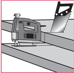
**Cutting panels:** Using a handsaw cut panel with pattern face upwards. When using an electric saw cut panel with decorative face downwards.
