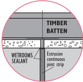
First trim off the tongues on the sides of each panel. Panels are easily cut on-site. The edges being covered by Reef panel extrusions. This will facilitate for faster installation. Panels can be joined together in continuous runs with decorative H joint extrusions.
