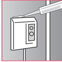
**Pipes and accessories:** Leave a 3-4mm clearance around all pipes and accessories and seal with a bead of Reef sealant. If a collar is to be fitted first seal with Reef sealant.
