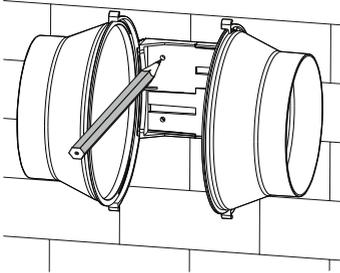
5. Fix frame to desired surface, using fixings suitable for wall type. Then replace central unit and bracing clips.
