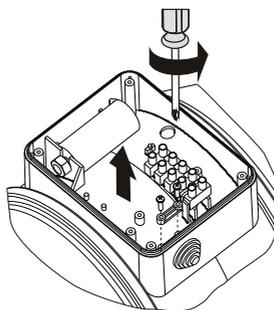
3. Feed cable through hole & replace grip.
