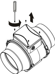
2. Using a screw driver, remove cable grip.
