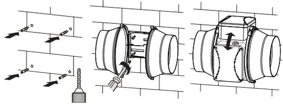
6. Connect the flexible ducting to both sides of the Inline fan with the metal hose clamps. Ensure there is a minimum of 1m straight ducting between fascia and fan.
