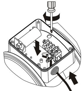
4. Wire the fan as per fig. C below.
