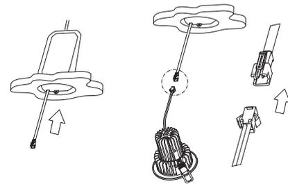
5. Push back the springs and push the lamp into the hole to fix in place. Please note the light fixture & driver must not be covered with insulating material. **There should be 100mm of free space around the light fixture in all directions.**
