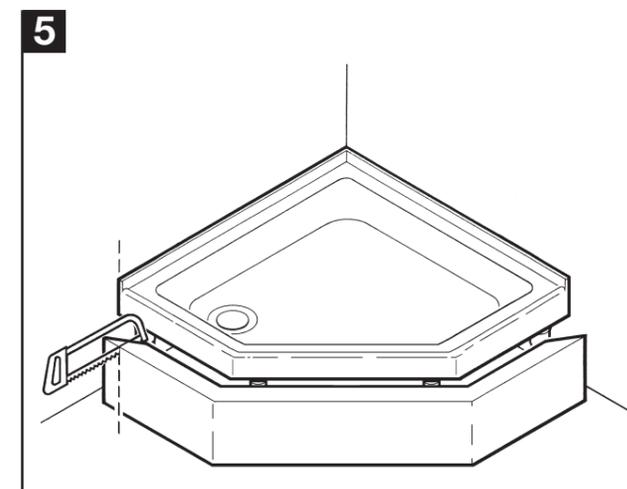
If necessary, carefully cut the outside edges of the panel to fit.
