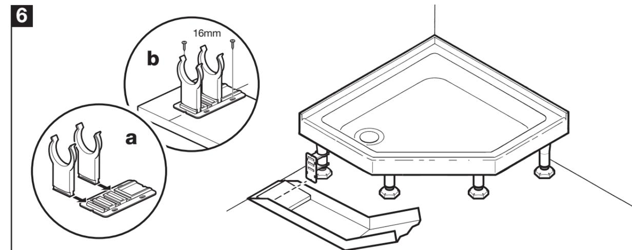
(a) Separate and assemble the panel brackets. Push fit the panel brackets onto the legs, align panel up with the brackets and mark the centre line of the brackets onto the back of the panel.
