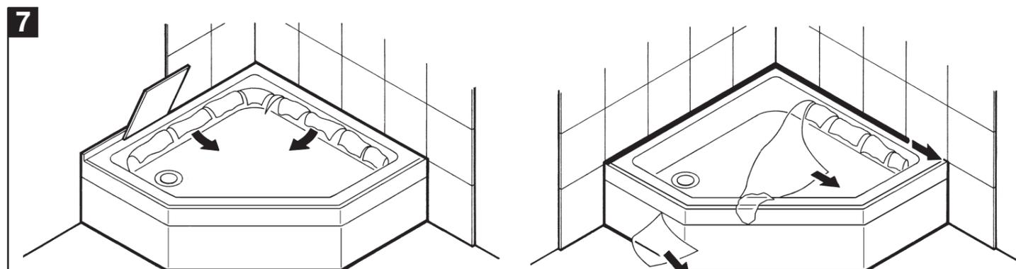
Peel back protective film from back edges of tray. **Tile over the upstands. Seal the wall edges of tray with silicone sealant.** When the final installation of the enclosure is complete, remove the remaining protective film.
