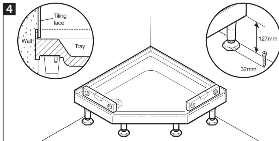
Ensure the tiling upstands are either recessed into the wall or boarded over so the tiling face is flush with the edge shown in the diagram. Adjust legs where necessary. Check tray is level in all directions (there is a built in fall on the tray for water drainage). Ensure all legs are wound down tight to the floor. Fix legs to the floor using 32mm screws, where accessible.
