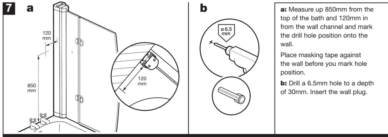
**a:** Measure up 850mm from the top of the bath and 120mm in from the wall channel and mark the drill hole position onto the wall.
