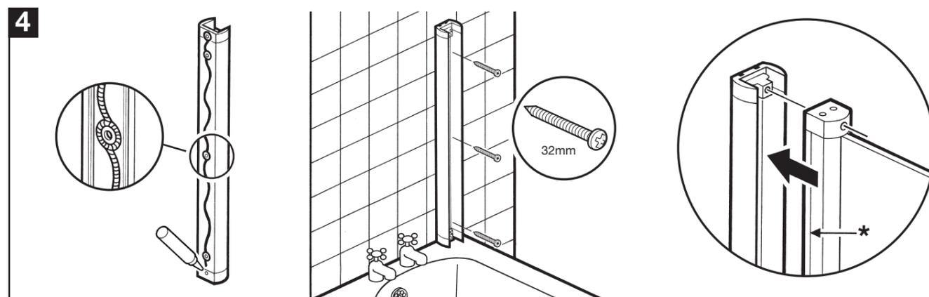
Apply silicone sealant to back of wall channel as shown. Fix wall channel to wall using the 32mm screws.
