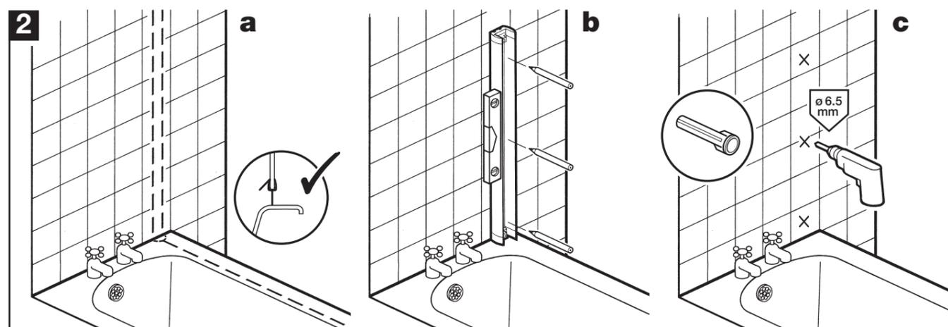
**a:** Position the fixed panel and bathscreen as far towards the inner edge of the bath as possible while being supported on the bath rim.
