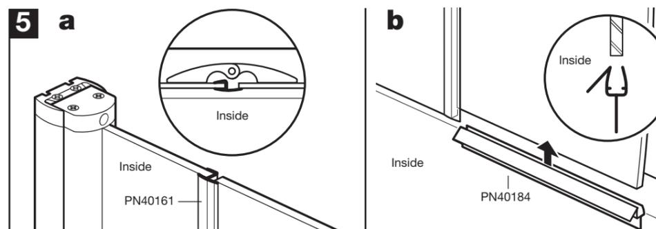
**a:** Push fit the vertical seal onto the edge of the fixed panel with the 'flap' on the inside of the screen. Trim to length if required.
