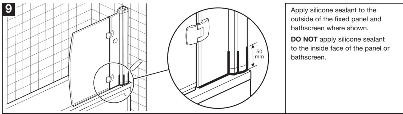
Apply silicone sealant to the outside of the fixed panel and bathscreen where shown.
