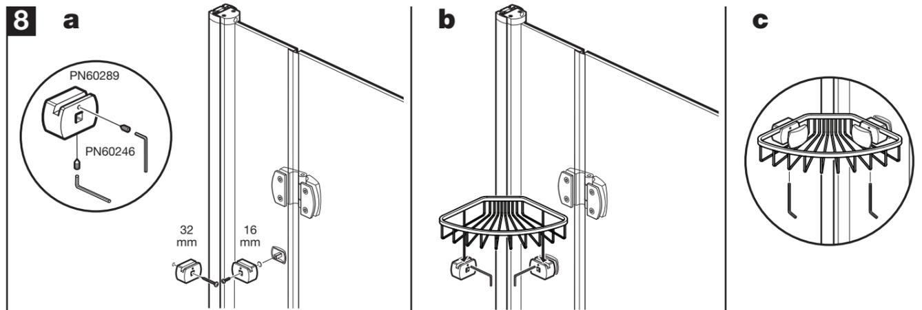
**a:** Partially insert grub screws into both brackets. Attach a bracket to the fixed panel, fixing through the bracket into a bracket cover using the 16mm screw, **do not over tighten**. Fix the remaining bracket to the wall using a 32mm screw, do not over tighten. **b:** Position the basket down onto the brackets and tighten the grub screws. **c:** Push on the bracket covers and tighten the grub screws from below.
