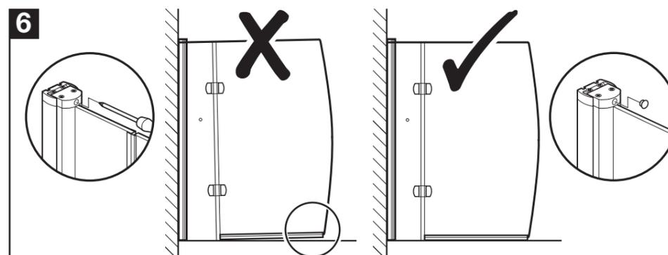
Adjust the bathscreen by tightening or loosening the screw at the top so that when opened, the bottom seal gently brushes the bath rim evenly along its length.
