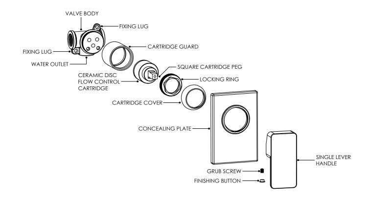
Components List (Twin Outlet with Diverter)
