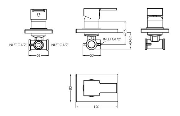
Key Dimensions (Twin Outlet with Diverter)
