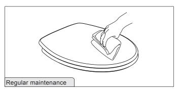
Clean the seat and hinge plates with a mild detergent then dry with a soft cloth.
