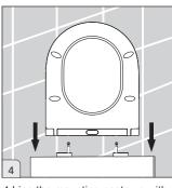
4.Line the mounting posts up with the holes in the hinge section of the seat and click into place.
