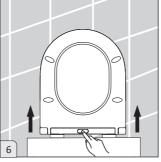
6.To remove the seat press the quick release button and lift off.
