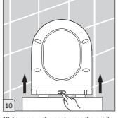
10.To remove the seat press the quick release button and lift off.
