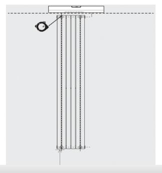
Allow enough room for the installation of valves or thermostatic controls
