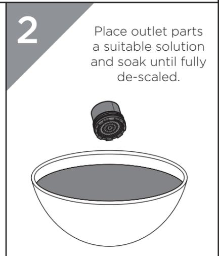
Place outlet parts a suitable solution and soak until fully de-scaled.
