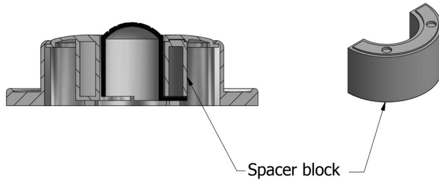
5. Align the rest of the button on top and press both buttons to test if they compress fully. Hold the large button fully compressed and mark the centre of the 3 mounting holes.
