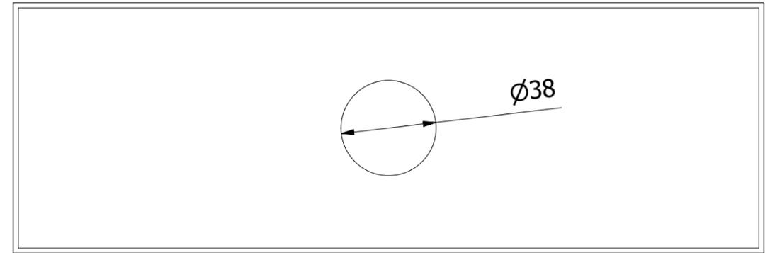
2. Insert base button into hole and align the 1 dot button to the right hand side. Secure base button with lockring, this can be used either way up depending on the thickness of the surface you are connecting the button to.
