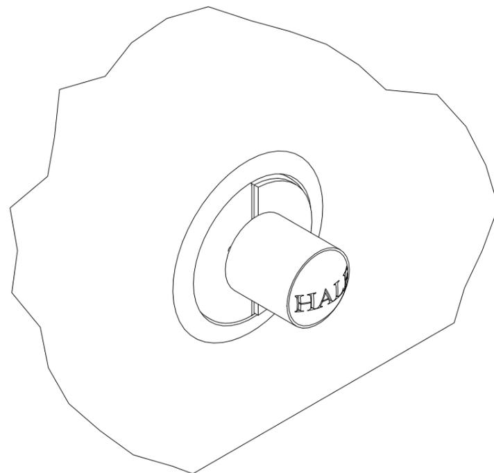
6. Attach the button using screws appropriate for the base material.
