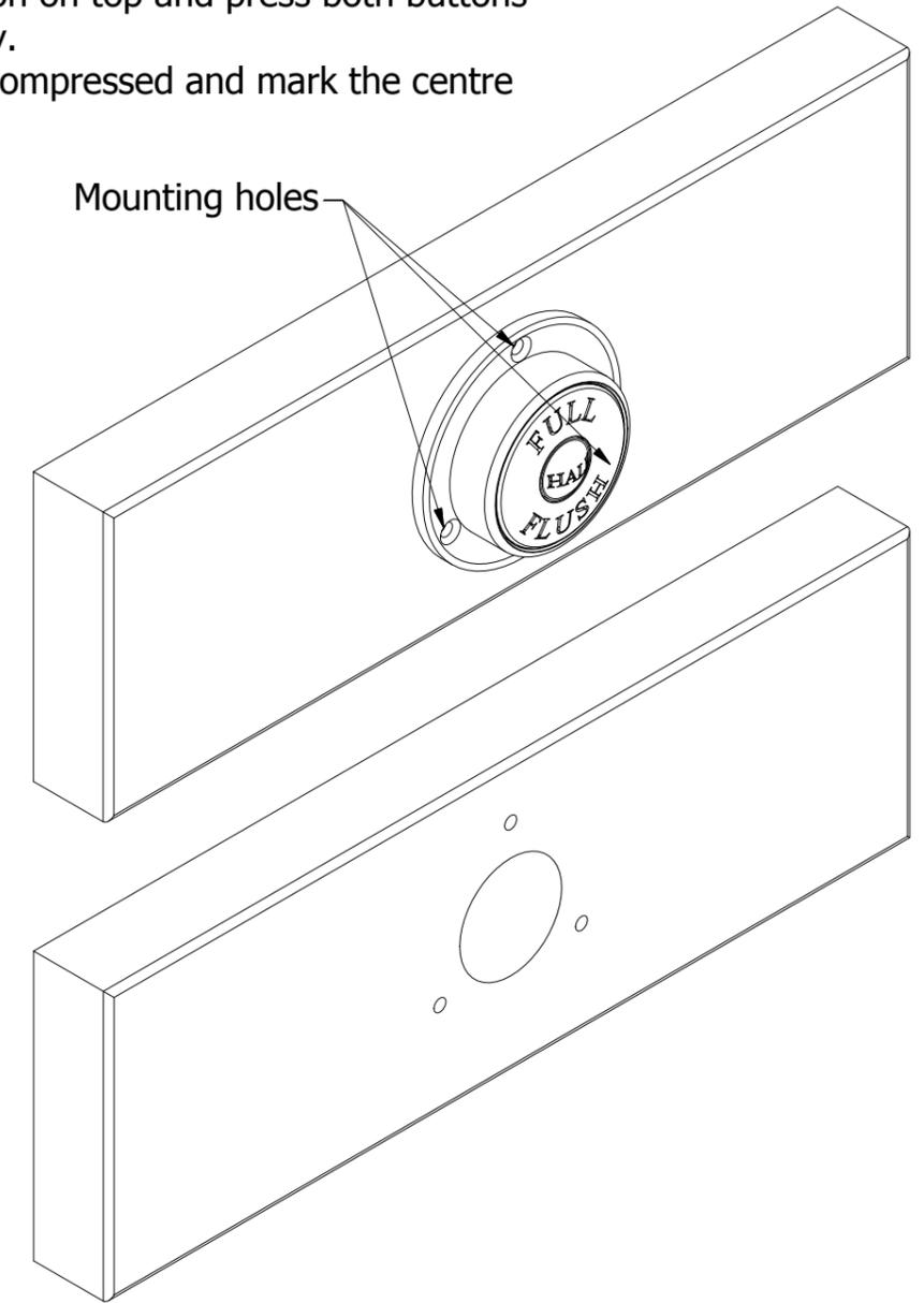
4. Using silicone adhesive, or double sided tape, stick the "half" button onto the one dot button as shown in the image. This aids alignment in the next steps
