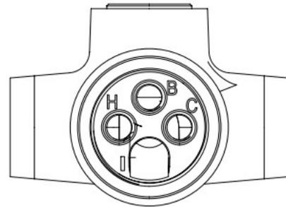
Feed the tails through the barrel thread and hand tighten into the tap. Fit the tap in the desired location using the locking nut and accompanying screws.
