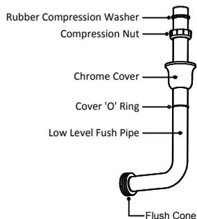
2. Put the parts labelled onto the flush pipe according to the diagram.
