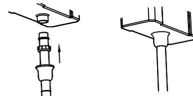
3. Insert the flush pipe into the bottom of the cistern and tighten the compression unit. To ensure a water tight seal use PTFE tape.
