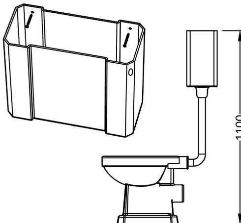
1. Mount the Cistern to the wall so that the top of the cistern is 1100mm off the floor. Secure to the wall using fixings suitable for the installation at hand (not supplied).
