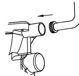
4. Insert the flush pipe and flush cone into the inlet hole on the Pan. Ensure the pipe is fitted securely into the Pan. Use a small bead of silicone to hold the cover in place.
