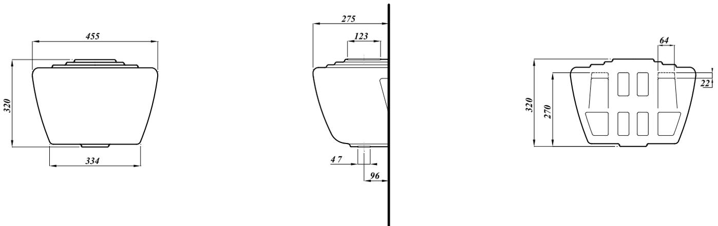
All dimensions are approximate and subject to normal ceramic variation. Although every effort is made not to change the above product specification. Changes to technical detail may be made without prior notification where necessary.
