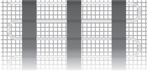
Mats are faster to install and have a fixed cable space that gives a pleasant even spread of heat over the floor surface. Caldo is powerful at 150w per square metre and is designed for general floor warming.
